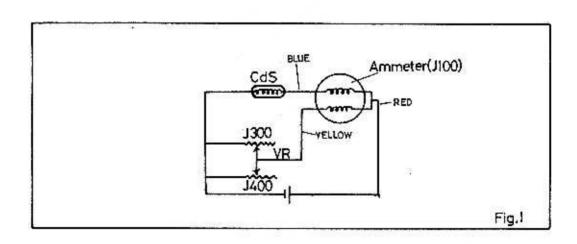
When the current value of CdS side becomes larger than VR Cds何の電流がVR側より大きくなると、 side, the needle of Ammeter (J100) goes up.
