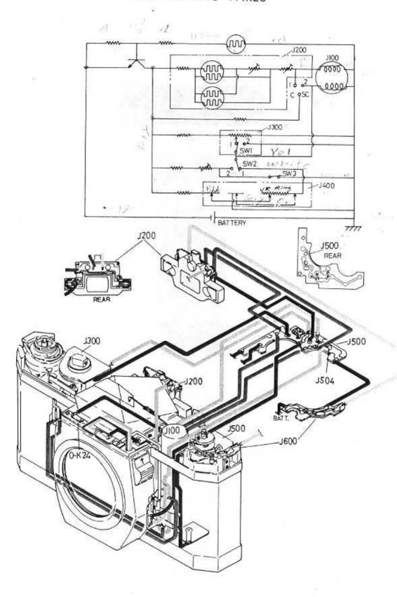
Product No. 23110 ASAHI PENTAX SP F Adjustment of mechanical exposure time, as mentioned before, is basically the same with that of SPOTMATIC (Product No. 23102). After exposure time is adjusted mechanically, electronical exposure time is adjusted with the adjustable resistors installed in print pattern assembly (0-T1).
