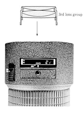
• Incorporate the 3rd lens group by using the tool J11195A.
