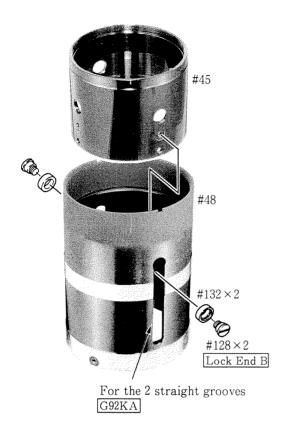
• Insert #45 into #48 and mount the guide ring in the best operative position.
