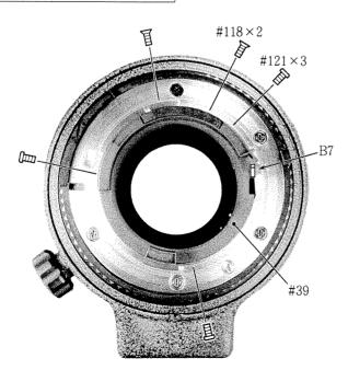
Mount the rear cover ring #39 to be the full aperture range of the aperture lever B7 (3.1<sup>+0.1</sup><sub>0</sub>).
