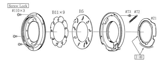
Inspection: Move #21 and B5 and check the operation of the aperture blade.
