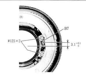
• By loosening the screws #125 (2 pcs.), adjust the position of the aperture lever B7 to be within the standard,  $3.1^{+0.1}_{0}$ , so that the aperture diameter may be proper when set to "full". At the same time, adjust the lateral position of the lever not to contact with the bayonet mount and rear cover ring. After adjustment, fix the screws #125 (2 pcs.) with the screw lock.
