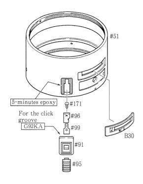
Caution: When incorporating, move the distance scale ring in the arrow direction because #96 may contact and damage it.
