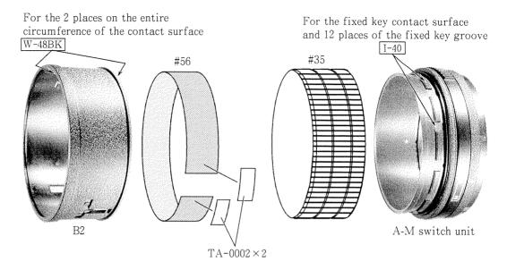
Inspection: Turn the MF ring and check the operation.
