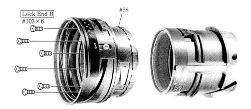
Caution: Don't adhere the grease of the gear ring to the encoder of FPC when incorporating the front lens group chamber unit.
