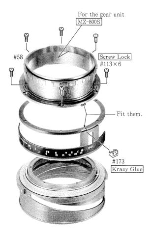
• Fit the groove of the focus distance ring #22 to the convex of the gear ring #58 and then adhere the stopper rubber #173.
