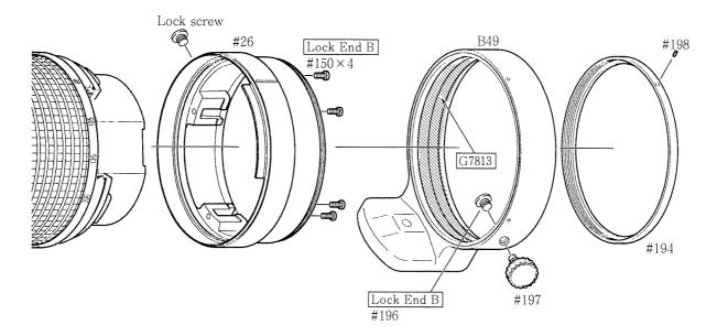
• Fit the lock groove of the tripod socket to the lock screw and then incorporate it.
