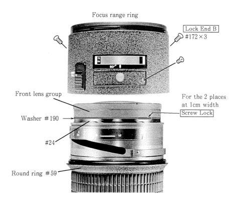
7 Mount the focus range ring. Attach the lock end B to the screw #172 (3 pcs.).
