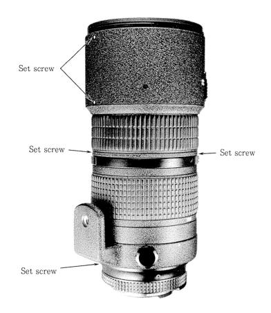
• Apply the black polishing paint to the heads of the set screws #168 (3 pcs.), #169 and #196.
