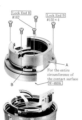
• Adhere the AF contact FPC to A and B of the fixed barrel #82.
