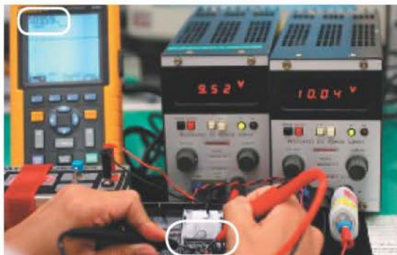
Make sure 10V is supplied to the tool battery.
