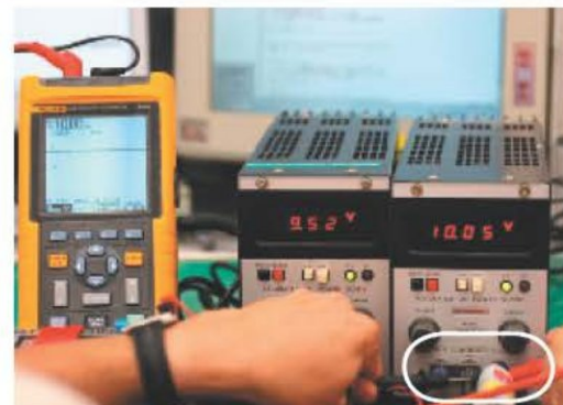
Measure the voltage between the electrode sections (+ and -).
