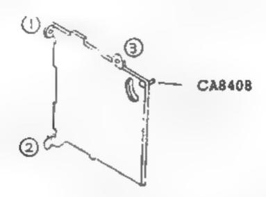
CA8408G (Pin) should be at 5.53 ± 0.05 from surface of the flesnel lens. Use the measuring tool KC-CA8408G. If the appropriate value is not obtained, adjust tightness of screws.
