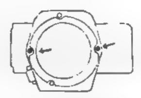
Pemove CA8944 String from adhered part of CA8980 (Pulley). Then comes off CA8880 (Gear). In case of such a type of repair that will require removal of CA8944 adhered to CA8980 (Pulley) only and not that of CA8877, CA8878, and CA8880, it is advisable to take following measures so as to insure that the CA8944 will not be entangled or become off position.
