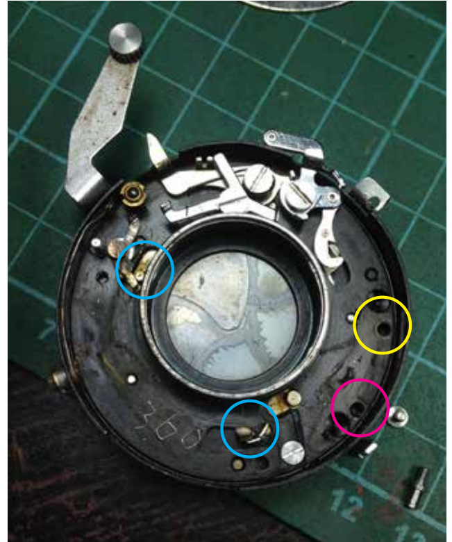
12: Now the big mechanism is gone you can see the smaller lever and pivoting parts on top. I HL the position here of the mechanism. This is where you can test of the blades by moving the lever points HL in blue. If yes, it is a good sign and it just needs cleaning up. Mine is stuck up so I must proceed further than this stage here.
