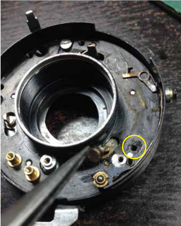
21: Remove the screw and take note of the spring position.
