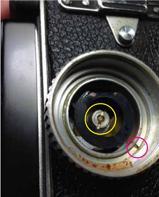
06: This is where you need a bit of ingenuity, the middle part with a slotted center HL in yellow, you need to loosen. Take note of the position of the slot in the knob HL in red. This is your guide for the infinity mark.
