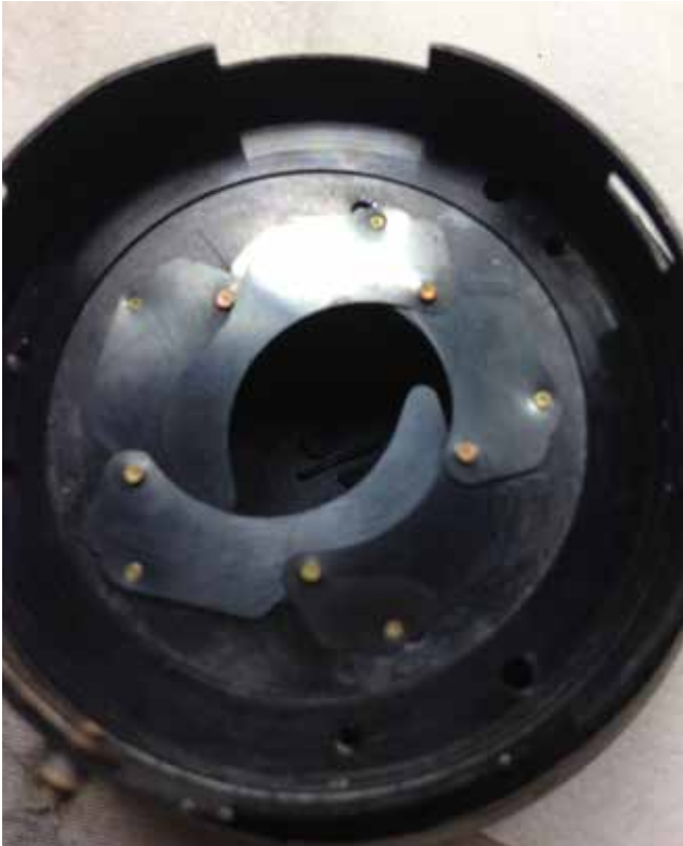
11: Once you get to blade #4 & #5 it gets trickier. Because you need to make sure that #4 & #5 goes below number 1. As you can see, the blades here are flipped. This is my first attempt and after trying to put it back it doesn't open & closed. So I re-started. Do note never touch them with your bare fingers. If you did, wipe them with fluid. Use tweezers or toothpick to move blades around.
