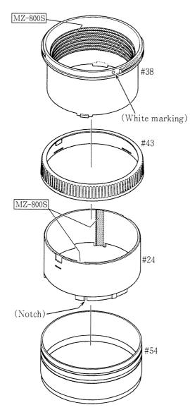
• Set to mount #38's white marking position and #24's notch position as shown in the left figure.
