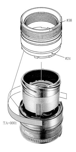
Peel off the tape TA-0001, and then remove the helicoid ring and the MF ring unit.
