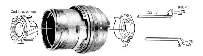
Caution: Due to already aligned 2nd lens group including G5 to G8 and the aperture blade housing, the 2nd lens group is set as a combined unit.
