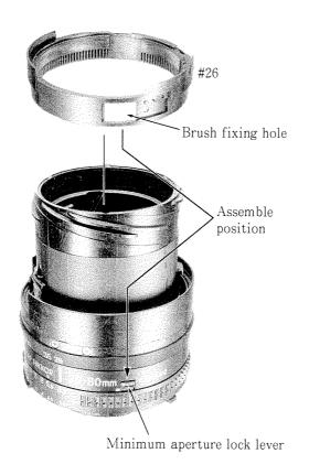
• Mount and set #26's brush fixing hole to meet the minimum aperture lock lever position.
