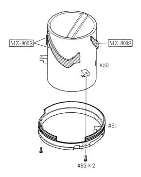
• Apply MZ-800S to 6 internal grooves inside the cam ring #50.
