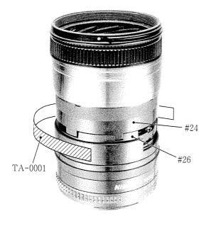
③ Fix #24 and #26 together by applying a tape TA-0001.
