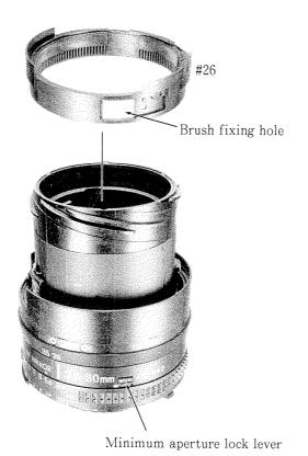
• Drive #26 and then set the brush fixing hole to meet the position of minimum aperture lock lever.
