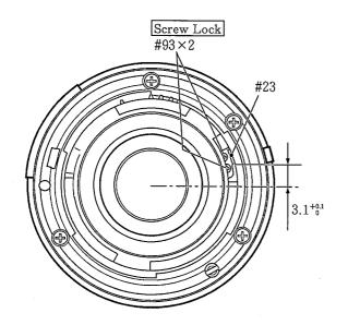
Unfasten screws #93×2 to adjust the position of the aperture lever #23 so that it comes into the rated value of  $3.1^{+0.1}_{0.0}$  to bring the aperture diameter whitin rated value at full aperture.
