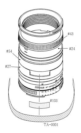
• Fix #54 and #27 together by attaching a tape TA-0001.
