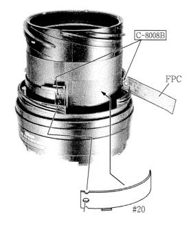
④ Attach #20 on where as shown in the left figure and then attach FPC on it.
