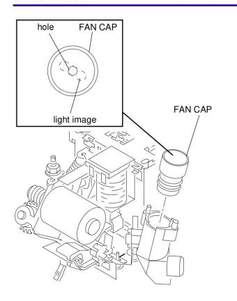
[11] Install the FAN CAP 232729 in the PHOTOCELL HOUSING.
