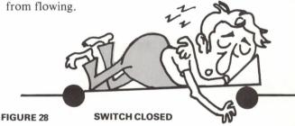
The simple switch we've been looking at here is called a single pole, single throw switch. Single pole, single throw is often shortened to **spst**. We'll be taking a detailed look at switches soon.
