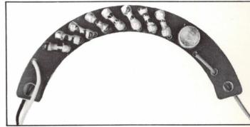
FIGURE 58 Metal film resistors used in a camera circuit.
