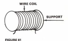
Construction of a wirewound resistor
