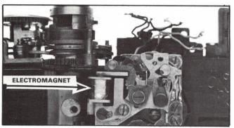
FIGURE 74 An electromagnet used to time exposures in a Copal Square shutter.
