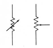
Schematic symbols for variable resistors FIGURE 62
