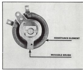
FIGURE 63 A wirewound variable resistor.
