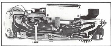
FIGURE 82 A gas filled lamp used to indicate a charged capacitor.
