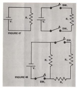
For example, in the circuit containing many resistors, each resistor would be identified by the letter R. Following the R identifying the component as a resistor would be a number: 1, 2, 3, 4...this number is called a **subscript**.
