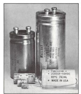
FIGURE 68 Electrolytic capacitors.
