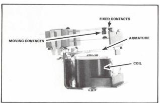
FIGURE 85 The parts of a relay.
