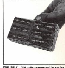
FIGURE 42 340 cells connected in series to make a 510 volt photoflash battery.
