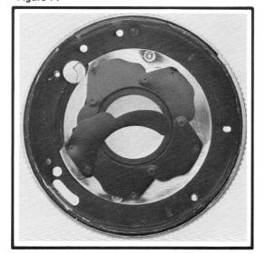
Now seat the first leaf as shown in Fig. 69. The downward-projecting pin must fit into the long slot in the diaphragm-control ring. Slide the leaf so that the pin is at the top of the slot, Fig. 69.
