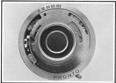
But, when you release the shutter, the pallet-control tab moves toward the inner edge of the pallet-control slot. This movement brings the pallet into engagement with the star wheel.
