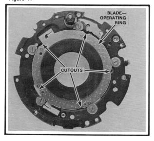
To align the cutouts with the washers, you must rotate the blade-operating ring to its fully counterclockwise position (as seen from the bottom, Fig. 44). But one part now prevents you from rotating the blade-operating ring fully counterclockwise — the stop plate on the other side of the mechanism plate, Fig. 45. During normal operation, the stop plate prevents the blade-operating ring from rotating too far counterclockwise — so far that the cutouts align with the washers.
