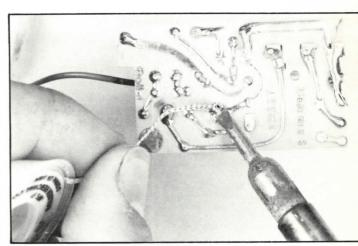
FIGURE 57 A desoldering wick in use.
