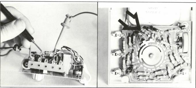
FIGURE 3 A clip-on lead provides an extra margin of safety.
