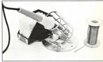
FIGURE 44 A soldering station.
