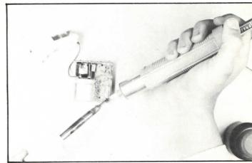
FIGURE 58 Using a vacuum pump to desolder.
