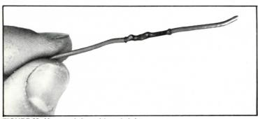
FIGURE 63 Heat and the tubing shrinks.
