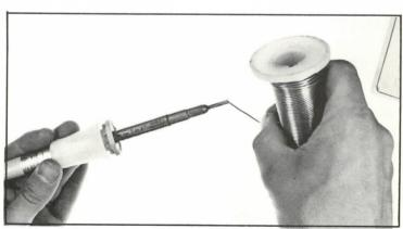
FIGURE 48 Steps in tinning an unplated tip.
