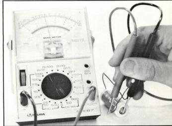
FIGURE 17 Using the milliammeter to measure a lamp's current.
