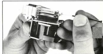
FIGURE 27 A contact burnisher being used to clean unplated contacts.
