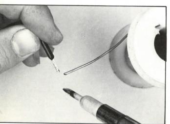
FIGURE 54 Tinning a stranded wire.
