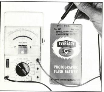
FIGURE 22 Using the high voltage scale to measure the voltage of an electronic flash battery.
