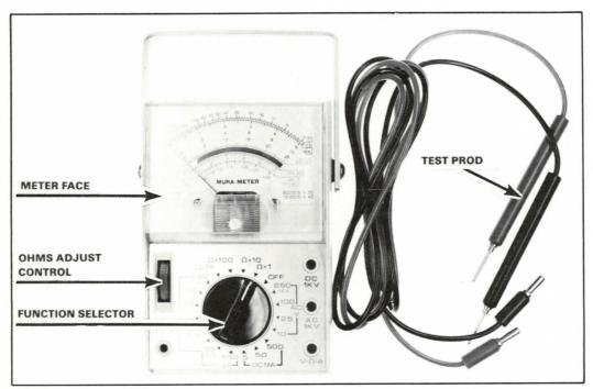
FIGURE 1 The volt-ohm milliammeter.
