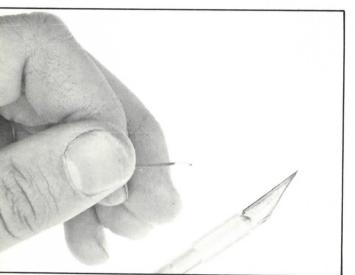
FIGURE 53 An angled cut is especially important with fine wire.
