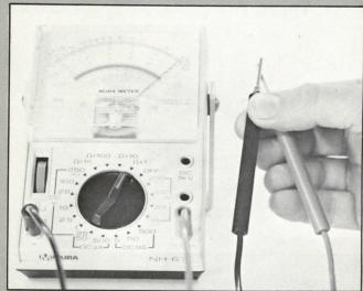
FIGURE 8 Zeroing the ohmmeter.
