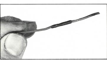
FIGURE 62 Slip tubing over the connection.
