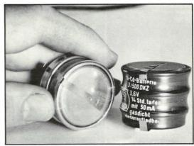
FIGURE 33 Replacement rechargeable batteries.
