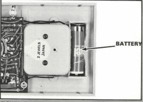
FIGURE 12 The internal battery used by an ohmmeter.
