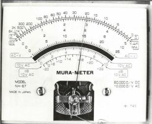
FIGURE 10 Reading 20 ohms.
