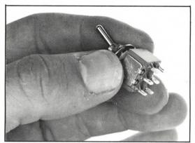
FIGURE 37 This is a double pole, double throw switch.
