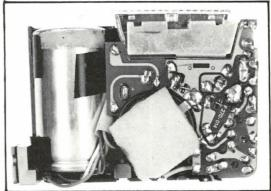
FIGURE 55 A compact electronic flash using a printed circuit.
