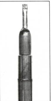
FIGURE 51 Tinned tip ready for use.
