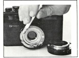
FIGURE 26 A pencil eraser safely cleans plated contacts.
