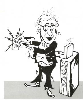
You'll often use your VOM to make measurements in circuits operating at high voltages. To avoid the possibility of a severe electrical shock, *never* hold a test prod by its metal tip. Always handle the test prods by their plastic insulators. As an additional safety measure, you may wish to use clip-type leads so that you may handle only one meter lead at a time.
