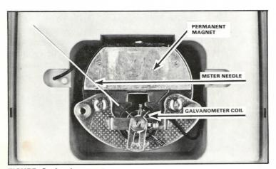
FIGURE 2 A galvanometer.
