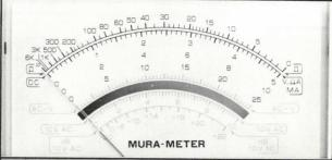
FIGURE 11 Reading infinite ohms.
