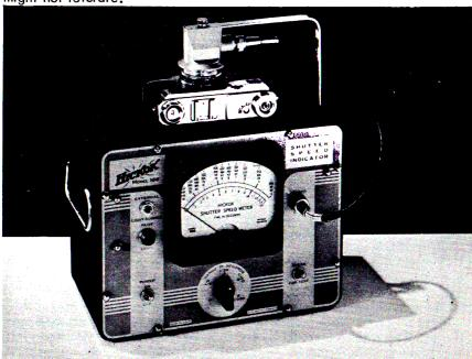
The Hickok Shutter Speed tester. Probably the first instrument of its type integrating light passage and reading in shutter speed.
