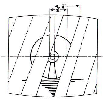
Test with 4 X 5 Graphic focal plane shutter set at  $\frac{1}{80}$  sec. exposure =  $\frac{.625^{\circ}}{8.75 \times 60}$  = .0119 secs. =  $\frac{1}{83}$  sec.
