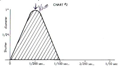
This graph illustrates the blade movement of an <u>average</u> shutter <u>opening and closing</u> within 1/100 sec. The cross-hatched <u>area</u> is about half of that in Chart 11, indicating an <u>exposure</u> of approximately 1/200 sec.
