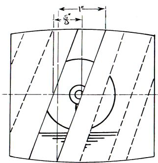
Test with 4 X 5 Graphic fecal plane shutter set at  $\frac{1}{90}$  sec. exposure =  $\frac{.625}{1^8 \times 60}$  = .0105 secs. =  $\frac{1}{95}$  sec.
