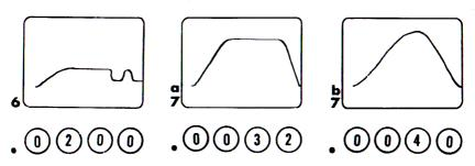
Shutters with blade bounce can be detected merely by stopping the diaphragm down as far as it will go and choosing a sweeptime 7 or 8 milliseconds longer than the total operating time of the shutter. Trace 6 shows the graph produced by a shutter having shutter blade bounce.
