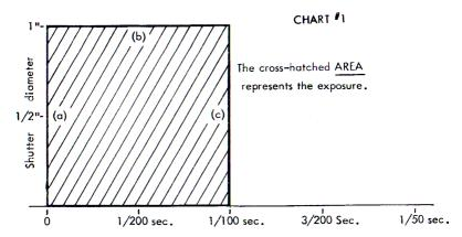
This graph illustrates the movement of the shutter blades of a one inch diameter shutter giving a perfect exposure of 1/100~sec.
