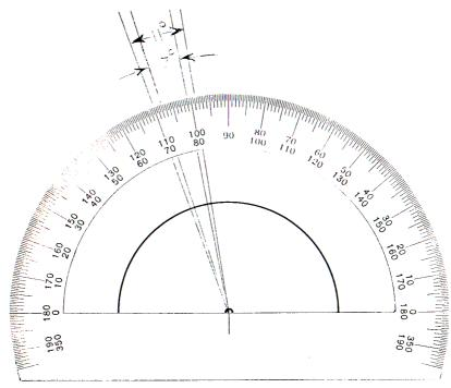
\$\$^2\$ The calculation for a typical shutter speed test width of blur:  $11^0 - 4^0 = 7^0$  (subtracting width of mark shown in Figure \$1\$). Opening and closing time (subtracting fully-expessed width from total width):  $11^0 - 7^0 = 4^0$ . During opening and closing phases, shutter yields average of 1/2 exposure:  $2^0 = 1/2$  epening and closing time. Actual exposure:  $7^0 - 2^0 = 5^0 = 10.7$  ms or 1/91 sec. actual exposure.
