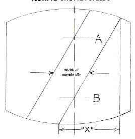
Some measurements used in a Focal-plane Shutter test. The Shutter moves "x" inches in 1/60 second.
