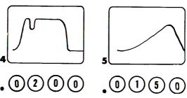
Trace 4 shows the graph traced by a shutter having poor leaf lever control. The trace illustrates that the shutter leaves open fully, bounce partially closed, and then reopen for the remainder of the exposure. Trace 5 illus-
