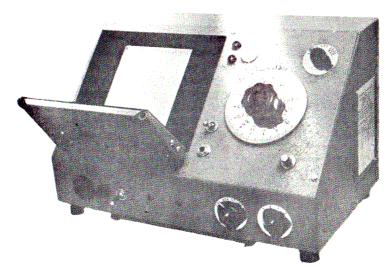
The Gardner Synchrotimer is a multiple-purpose instrument used for checking synchronization and shutter speeds. The calibrated delay is variable from 0 to 1200 milliseconds making shutter tests possible from 1/1000 sec. to 1 second. Standard model shown requires flash synchronization or cable release socket. Also available with photoelectric trip circuit which makes it valuable for testing shutter speeds of any shutter.
