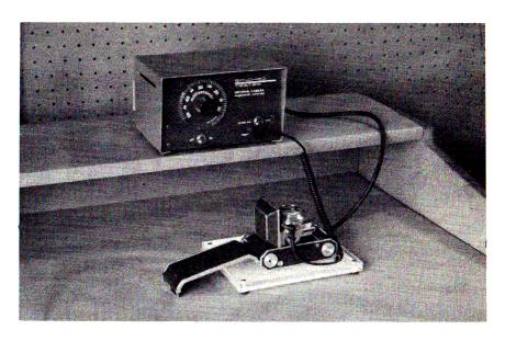
The ServiShops Synchrotester is a low-cost electronic "flash" type instrument most useful for testing synchronization. With some simple calculations it is possible to test shutter speeds (faster than  $1/25~{\rm second})$  of synchronized shutters, also.
