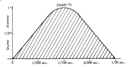
This graph illustrates the blade movement of a shutter operating more slowly than Chart 2 describes. The actual exposure delivered in this case is 1/100 sec., even though the total time involved is 1/50 sec.
