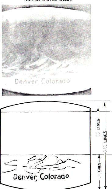
Because the shutter may start operating at any time, some of the scanned lines may appear at the top and some at battom of TV screen.
