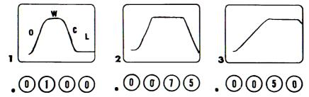
Typical traces produced by the Analyzer. Trace 1, upper left, analyzes a between-the-lens shutter with O indicating the opening time; W, the open period; C, the closing time. Trace 2 represents the same shutter after
