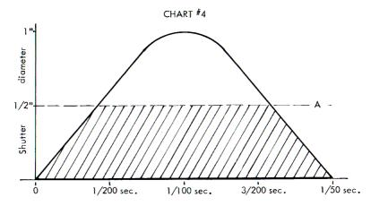
This graph illustrates the increase in exposure given by the shutter in Chart  $^{\#}3$  when the diaphragm is stopped down. The new exposure is approximately 1/66 sec.
