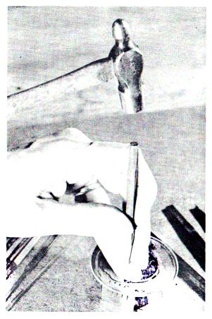
Swaging a speed cam to expand the metal. Lay the speed cam on a bench armil and carefully place the swaging punch in position adjacent to the area to be expanded. Choose an Choose a punch of the proper shape and size to avoid changes except where desired.
