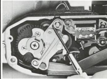
Figure 50 Replacing E-ring
