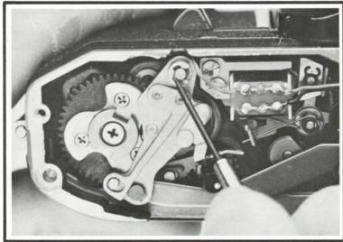
Figure 49 Removing E-ring
