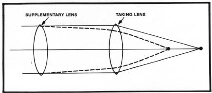
Figure 53 Positive supplementary lens decreases focal length.
