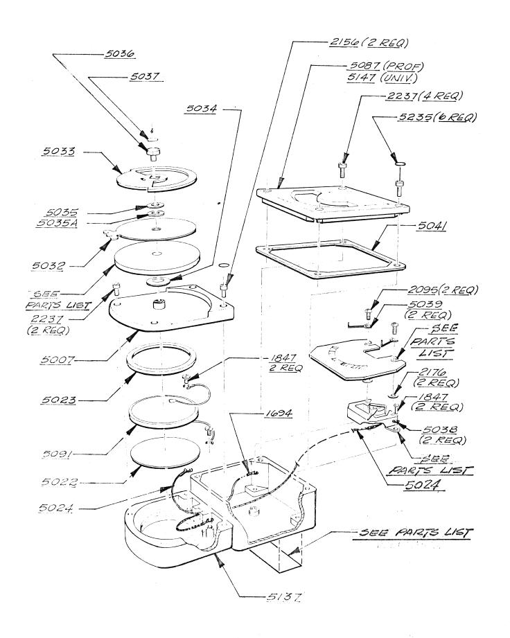
FIGUR<u>E II.</u> EXPOSURE METER EXPOSIBLICALL & "UMIVERSAL" (CURRENT METERS)
