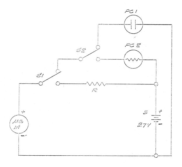
PCI VACTEC SELENIUM CELL-OUTPUT = 300 MQ AT 250 FC
