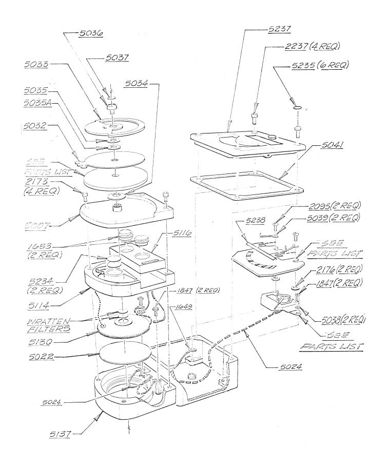
FIGURE II EXPOSURE METER "COMBI-500" (CURRENT MODEL)
