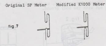
2. Also, because of the different design, the meter sensitivity will be slightly lower.
