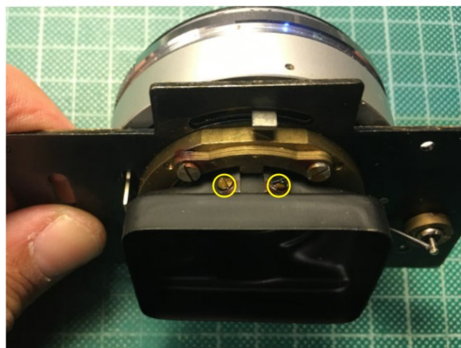
16.1 — Shutter/Focus panel with light cover
