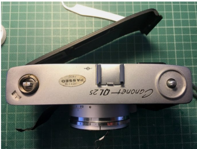
12.1 — Top cover without the cock and rewind lever
