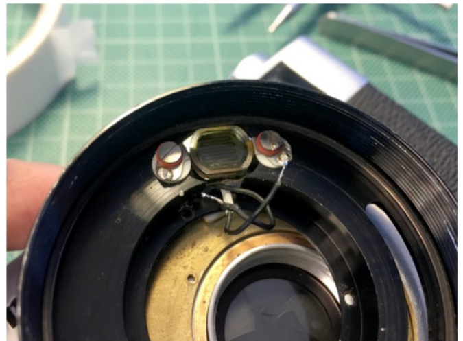
5.3 — Unweld the EE wires
