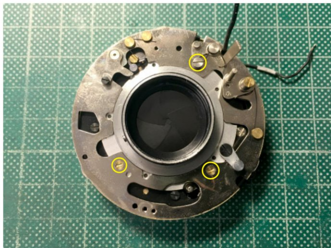
18.6 — Shutter/Diaphragm cover plate
