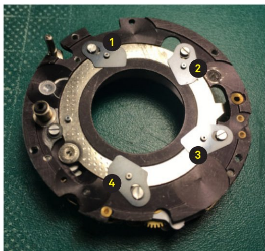
23 — Assembly of the shutter blades
