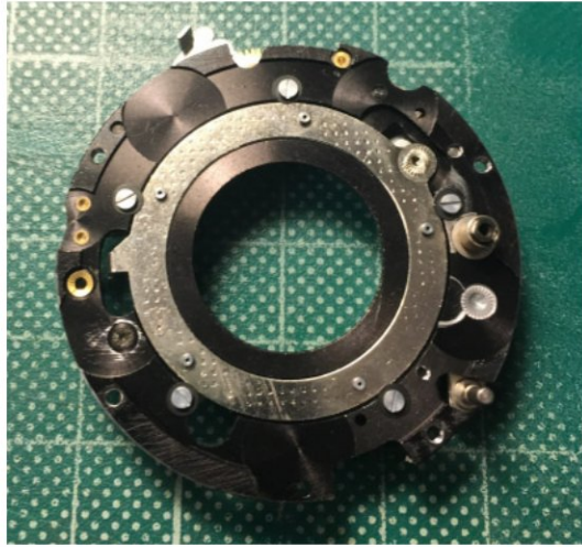
20.1 — Shutter plate, side of the blades
