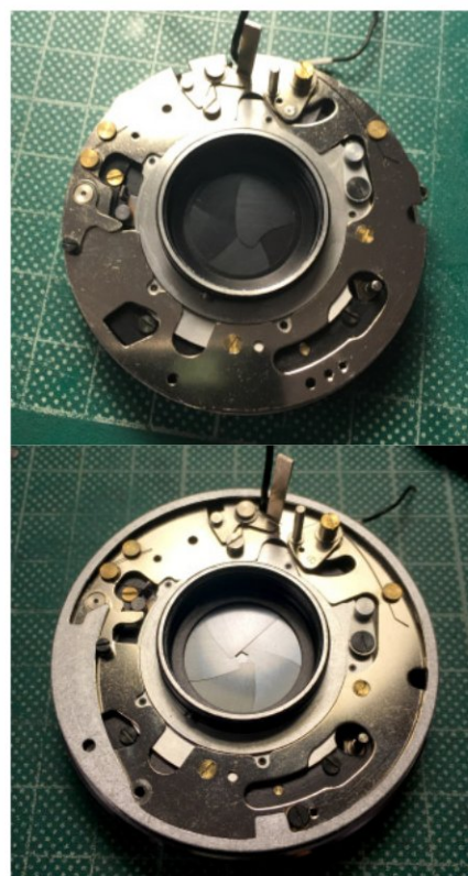
24 — Diaphragm plate/ring assembled
