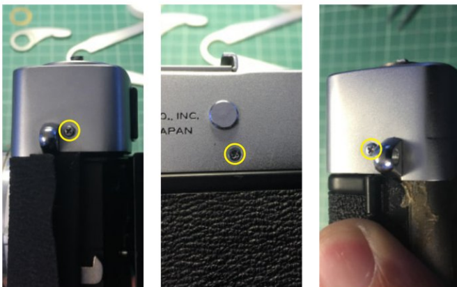
12.2 — Top cover, remove this 3 screws
