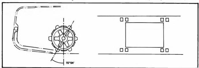
Figure 126 Sprocket position as seen from bottom of camera
