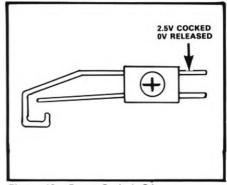
Figure 12 Reset Switch S1
