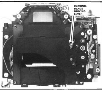
First section of opening blade in position Figure 79
