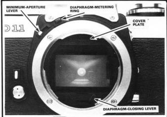
Figure 5 Figure 6 Front-plate/mirror-cage/shutter assembly
