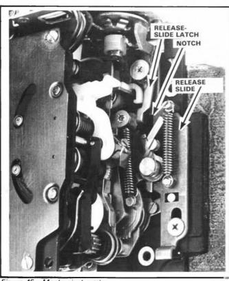
Figure 45 Mechanical setting
