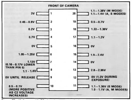
Figure 65 Voltages with S5 closed, shutter cocked
