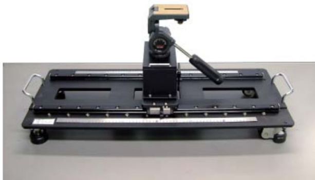
Slide rail for lens alignment equipment
