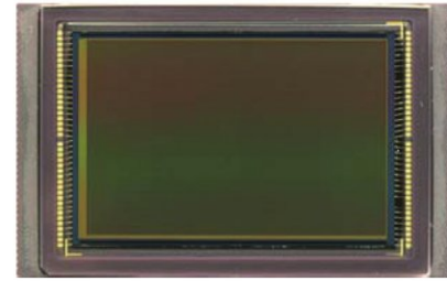
Fig. 001 Imaging sensor (actual size)
