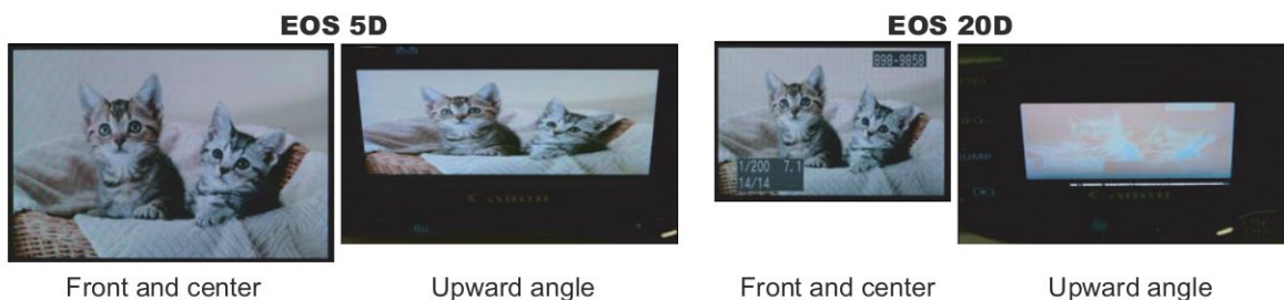
Fig. 026 LCD monitor viewing angle comparison
