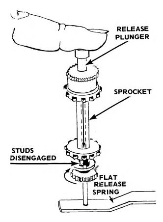
FIRST CURTAIN WIND GEAR IS FREE TO FIGURE 30 ROTATE (IN DIRECTION OF ARROW)
