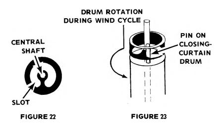
In the shutter-released position, the opening curtain holds its drum all the way clockwise (as seen from the top) — against the stop pin at the bottom of the camera. If there were no stop pin, the opening-curtain take-up roller could pull the opening curtain too far past the focal-plane aperture. In turn, the closing curtain pulls its drum all the way clockwise. The pin on the top of the closing-curtain drum is then against the end of the slot in the opening-curtain drum,
