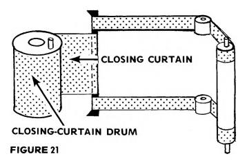
Usually, a screw or a taper pin holds the lower end of the opening-curtain drum to the shaft. So if you're assembling a drum, you'll have to remove the lower end of the opening-curtain drum. You can then insert the shaft through the hole in the center of the closing-curtain drum.
