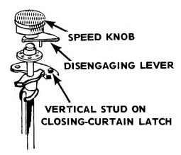
When you release the shutter, the speed-control plate turns with the opening-curtain drum. And the disengaging lever spins in the same direction. At the proper point in the opening curtain's travel, the disengaging lever strikes the vertical stud of the closing-curtain latch, Fig. 40. Exactly when the closing curtain releases depends on the position of the disengaging lever — how close it sits to the closing-curtain latch with the shutter cocked.
