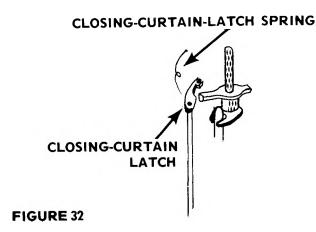
A long shaft riveted to the closing-curtain latch extends to the bottom of the camera. Here, it rests against the flat release spring, Fig. 33. Normally, the flat release spring holds the closing-curtain latch above the plane of the closing-curtain cam. So the closingcurtain cam may rotate freely with the closing-curtain drum from the released position, Fig. 34, to the "ready" position, Fig. 35 — it just passes under the closing-curtain latch.
