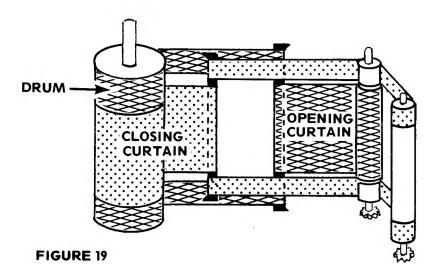
The drum winds both curtains at the same time. But it releases the curtains separately. Consequently, the drum has two separate sections — one section that controls the opening curtain and another section that controls the closing curtain. The unique construction of the drum allows both sections to turn simultaneously during the cocking cycle and separately on the release cycle.
