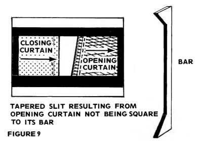
Apply a light coat of shellac or rubber-base cement (such as Pliobond) to the bars. Then, carefully align the curtains in position. While the cement is drying, you can make precise adjustments to the squareness of the curtains.
