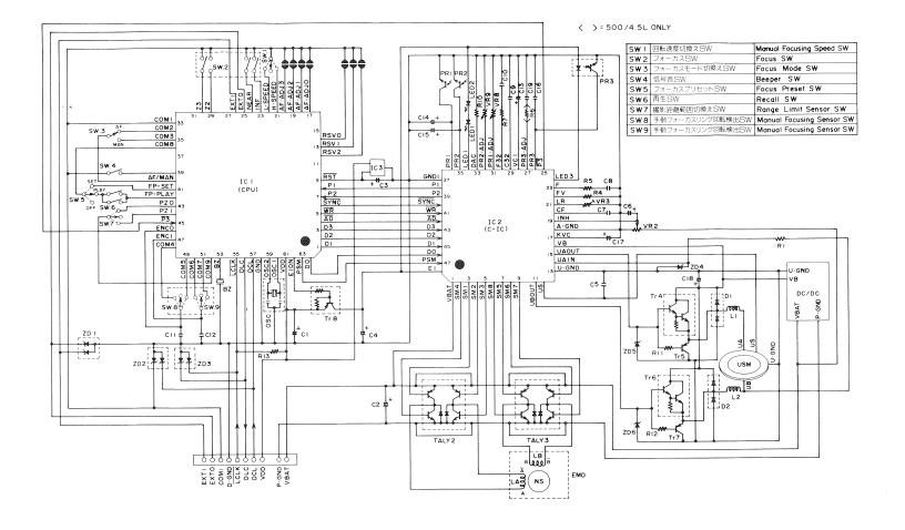
DC/DC converter is activated, and lens MPU receives VDD, lens DC/DC converter and VBAT (for the DC/DC converter). At this time, the lens MPU applies a low to the E1ON pin turning Tr8 on which supplies E1 to the C-IC.
