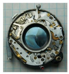
The mechanism at 7'oclock, stamped T.K., is the self timer.
