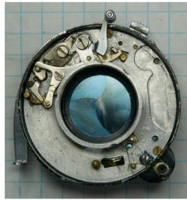
Mark the position of the flash sync port on the aluminum plate ... this will help when putting the shutter back together.
