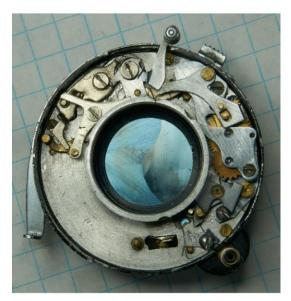
The slow speed escapement is held on by two large round headed screws. The top-middle one can be accessed after cocking the shutter to push some arms/gears out of the way.
