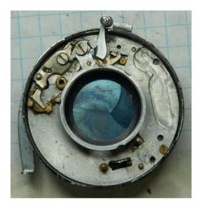
Remove the spring and sync post parts.
