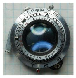
There are some small grub screws that hold the focus ring to the first lens element ... I could not budge them, so I worked around it.
