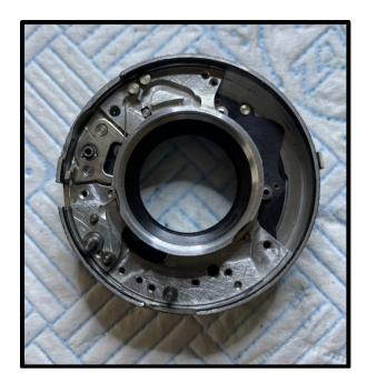
4. After cleaning, reinstall the leaf lever and reset the leaf lever spring.
