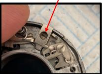
9. For the cleaning of the retard mechanism, I used an ultrasonic cleaner. The fluid was water with a little washing up liquid. I set the cleaner for 4 minutes. After this, the escapement was washed in clean water, before being submerged in Isopropyl and blown dry.
