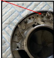
7. Clean and reinstall the cable release lever. This step is a little tricky as this lever needs to connect with the lug on the bulb lever, before being depressed onto its post.
