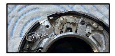
6. Clean and reinstall the bulb lever and inner release lever. Reseat the bulb lever spring on the cable release lever post.
