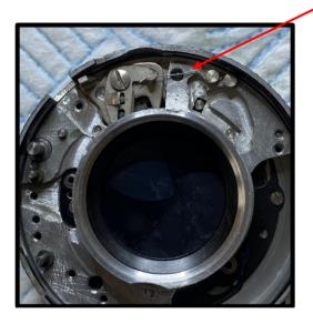
5. Clean and reinstall the high-speed spring.
