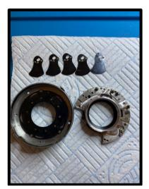
15. Remove the 3 cover plate screws which hold the blade operating ring in place. Note that one of the screws is longer.
