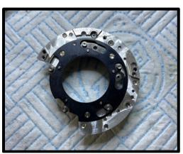
2. Install the shutter blades, starting with the first blade on the pins closest to the leaf lever, then working in a clockwise direction.
