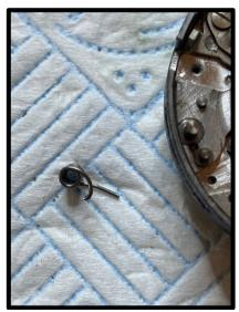
10. Disconnect leaf lever spring from its post on the leaf lever. The spring will stay attached to the mechanism plate. Remove leaf lever.
