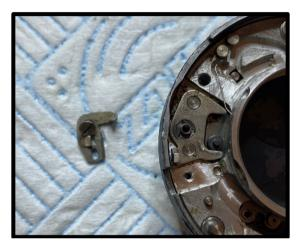
11. Hold down pallet lever and move the retard lever so it is locked towards the outer edge of the shutter. This enables the retard assembly to be removed.
