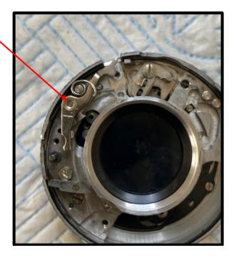
8. Clean and reinstall outer release lever and cable release socket.
