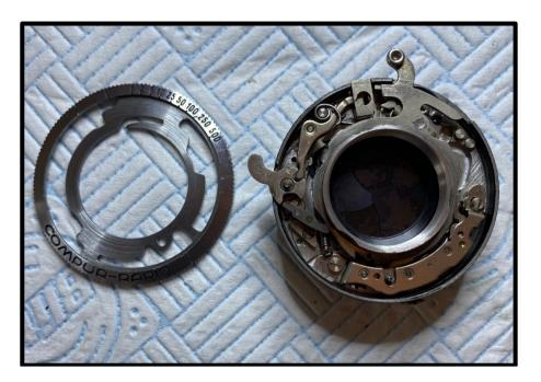
4. Next the main lever is removed. First, lift the setting lever a little and allow the spring tension to dissipate anti-clockwise. Then, disconnect the main spring from its stud at the end of the retard escapement mechanism.
