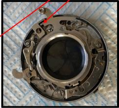
12. Now the retard section must be correctly positioned before being tightened down. Start with both ends towards the centre of the shutter, then back the retard lever end off slightly and tighten the screws. Test the action at this point, holding down the main lever to avoid it disengaging.
