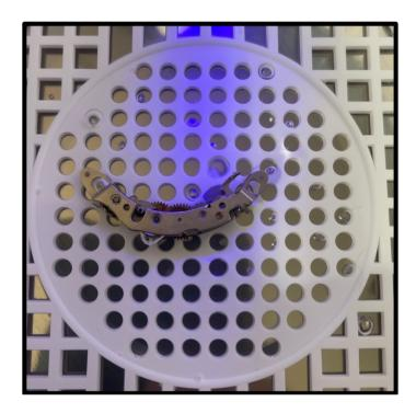
10. Lubricate the pivot points on the retard mechanism using Nyoil or similar. Reinstall the screws and main spring bracket but do not tighten.
