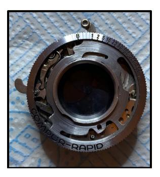
14. Clean and reinstall the nameplate. Lock it in place with the semi-circular cam. Clean and reinstall the aperture pointer.
