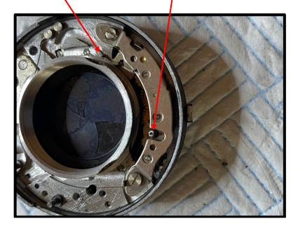
12. Remove the retard assembly retaining screws and main spring bracket, then lift out the retard assembly. Note the different lengths of screw.
