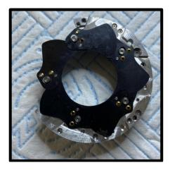
3. Reinstall the shutter housing with its 3 screws.
