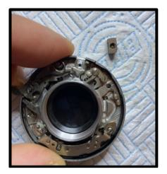
6. Prise the cable release lever from its post.
