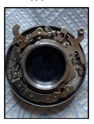
13. Clean and lubricate the bearing edges of the speed control cam. Reinstall it and check speeds seem good by ear (for example, check that 1/25 sounds faster the 1/10, the difference should be noticeable.)
