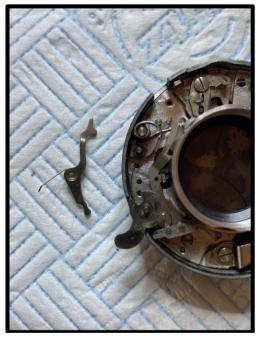
7. Disconnect the bulb lever spring from its position on the cable release leaver post so that it rests on the shutter housing. Remove the bulb lever via its screw and the outer release leaver by prising off its post.
