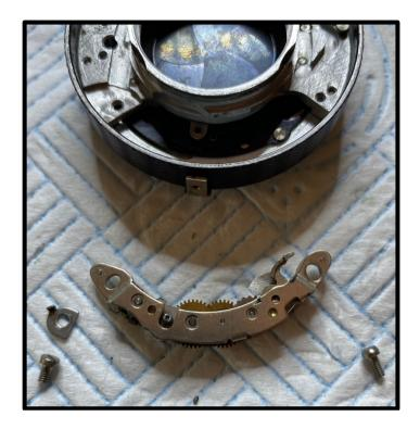
13. Move the blade operating ring stud until the shutter blades are fully open.
