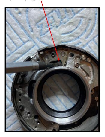
14. Turn the shutter over and remove the 3 screws holding the mechanism plate. Gently lift the shutter housing from the mechanism plate to revel the shutter blades. Remove the shutter blades.
