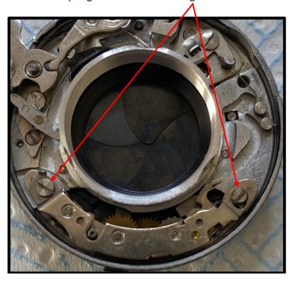
11. Next, seat the main lever and reattach the main spring to its bracket post (ensure the coils of the spring face downward from the connecting loop). Then rotate the main lever clockwise into its position against the main lever stop stud. It will be necessary to ease the leaver down past the pallet lever and inner release lever.
