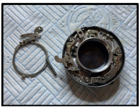
5. Hold the outer release lever so that the screw holding the cable release socket is accessible and remove this socket.
