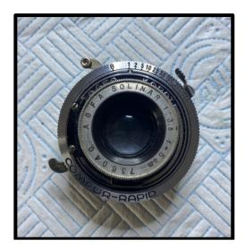
4. Loosen the 3 grub screws to free front lens element.
