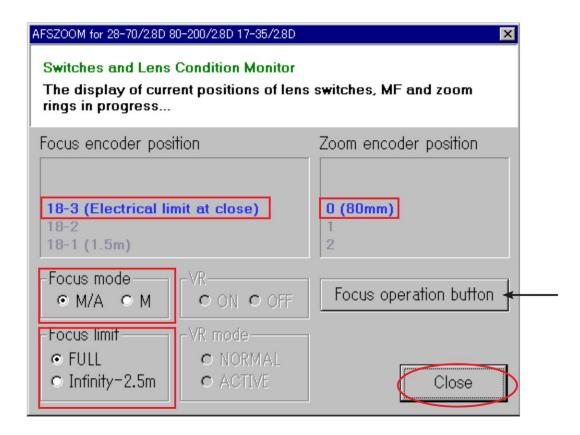
• Clicking the focus lock button of the lens changes the screen indication to the following:
