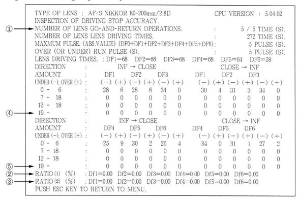
**Note**: If the MF ring is rotated during lens scanning, an error value is shown for the pulses. Don't touch the MF ring during operation.
