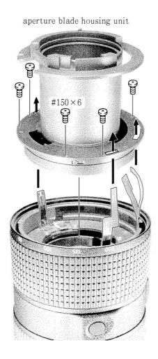
Note: For mounting and fixing the aperture blade housing unit, as instructed in the figure below, avoid to cut off the MR-FPC.
