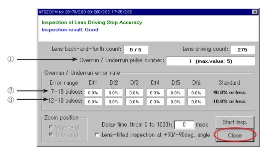
The number of overrun/underrun pulses must be within the standards after the lens back-and forth driving-motion five times.
