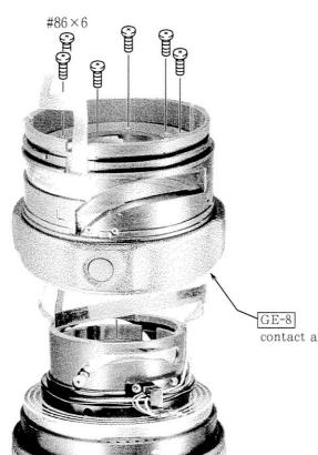
Note: Apply the Screw Lock to one piece of the screw #86 which is used for fixing to a white screw hole for the sake of earthing on the main lens body.
