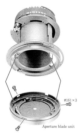
After mounting and fixing, operate the aperture ring and the aperture lever and check whether the aperture blade can interlock or not.
