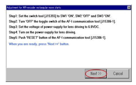
• With reference to ① - ⑤, make the adjustment so that the results become within standard. When the adjustment is completed, click "Adj.ends" to complete.
