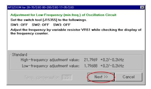
• By following the instructions on the screen, check the frequency adjustment value. If the result is not within standard, make the readjustment.
