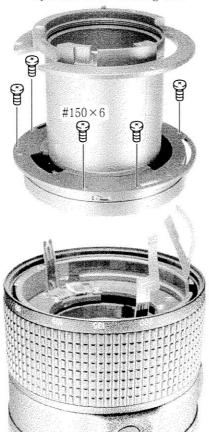
Caution: For removing the aperture blade housing unit, as shown below, avoid to cut off the MR-FPC.
