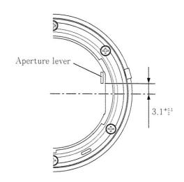
Adjust the position by loosening the screws  $\#80 \times 2$ . The aperture lever position must be within  $3.1^{+0.1}$  to obtain the proper maximum aperture diameter. After adjustment, fix 2 pieces of the screw #80 by the Screw Lock and then remove the aperture ring unit.
