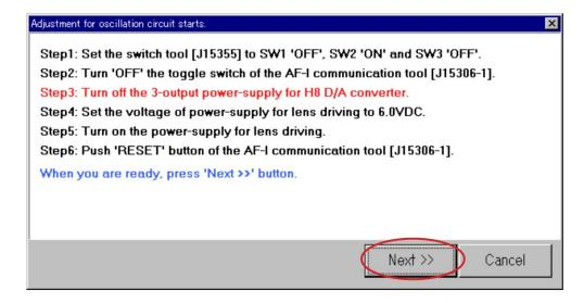
• By following the instructions on the screen, adjust high-frequency wave. When the adjustment is completed, click "Next".
