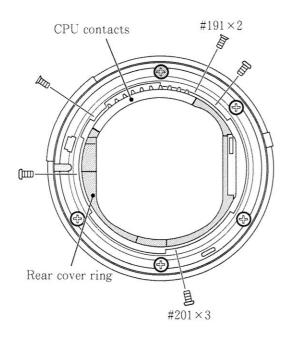
Caution: The rear cover ring can not be removed by removing 3 pieces of the screw #201 alone.
