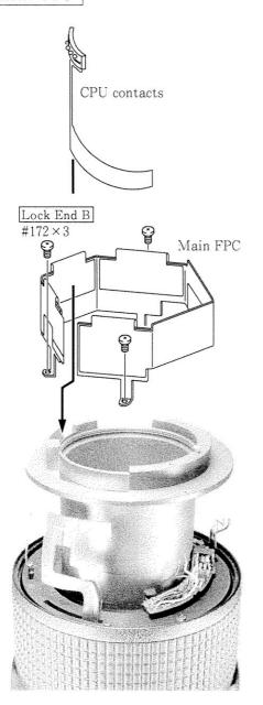
• Connect four connectors and solder each wire as shown below.
