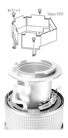
• Remove the four connectors and wirings described below.
