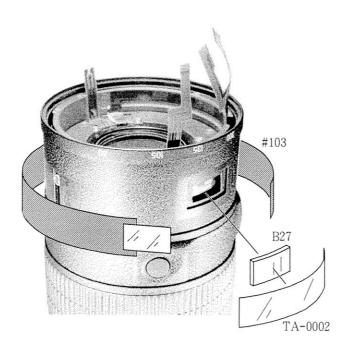
• After removing the rubber ring #37, remove the zoom encoder brush.
