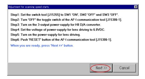
• When the toggle switch is turned ON, scanning drive starts. Make the adjustment so that the result becomes within standard, then "input driving frequency to be memorized".
