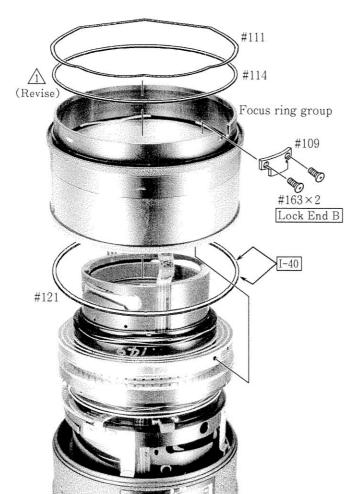
Note: Be sure that when mounting and rotating the focus ring, the focus index should follow the motion the focus ring makes, and as soon as the focus index touches the limit, the focus ring alone should rotate.
