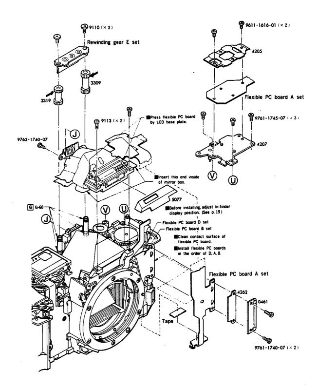
■After completion of assembling, solder lead wires referring Schematic Wiring Diagram on next page, and arrange the lead wires following Lead Wire Arrangement on p. 14.
