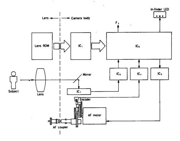
Auto focusing block is composed with three ICs (IC6, 7, 8).
