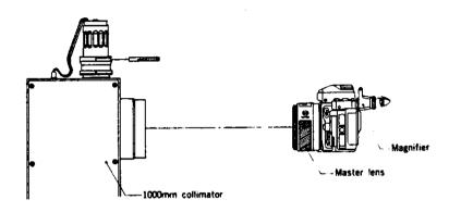
2. Make sure that the scale of master lens is positioned at infinity  $(\infty)$  and move mirror stopper up and down to bring chart image into focus. (See Fig. 2)
