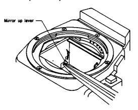
Lifting mirror up with tweezers, push mirror-up lever in the direction of arrow to keep shutter open. When shutter open, do not push mirror-up lever any longer; otherwise, M<sub>1</sub> will run idle.
