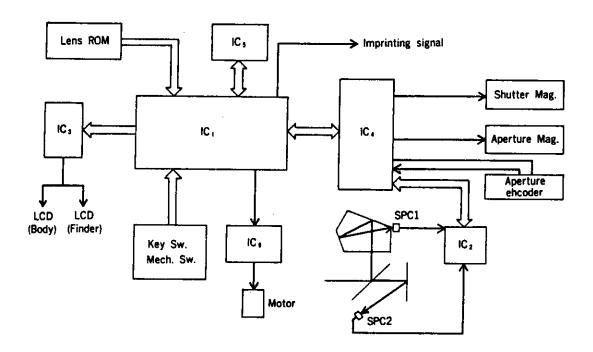
Metering Sw. ON → IC 1 starts to activate.
