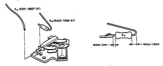
3. After soldering  $R_{51}$  on flex PCB-A, solder  $\ell_{43}$  on  $R_{51}$  reverse end. Solder leg of  $R_{50}$  on flex PCB-A. (See below fig.)
