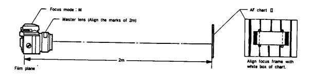
2) Turn touch switch (or metering switch) ON: low-contrast signal should be indicated (▶ ◀ blinking). If other focus signal than low-contrast lights, re-adjust AF following procedures ① to ⑧ since it shown AF area deviation.
