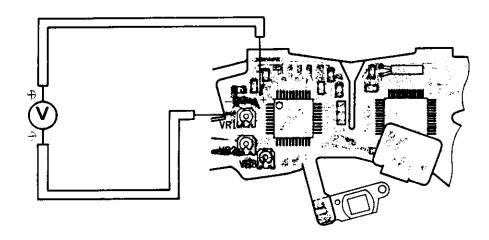
2. With main switch and measuring switch (or touch switch) turned ON, adjust by turning  $VR_1$  so that voltage is in  $1152\pm 5\,\text{mV}^*$
