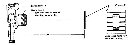
2. Turn touch switch (or metering switch) ON: Low-contrast signal should be indicated (⋈ blinking). If not, re-adjust and re-check AF area, following procedures from □.
