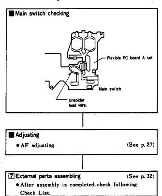
• Remove the lead wire which has been soldered for operation checking.
