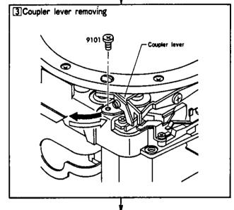
Remove screw (9101) and then remove coupler lever in the direction of arrow (➡).
