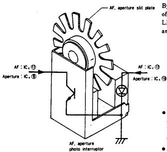
By slit plate rotation, light from LED to photo transistor is cut off repeatedly. Photo transistor outputs light/shade signal of LED. Light, received by photo transistor, is converted into pulse and input to IC<sub>1</sub>, IC<sub>5</sub> by IC<sub>4</sub>.
