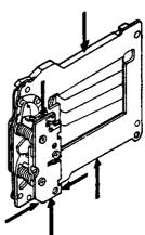
2. Fit © of new shutter set into body first, and secure it with two screws (9107).
