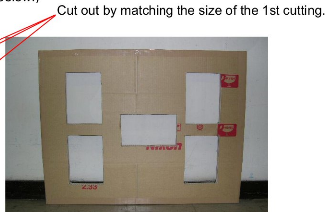
(Fig. 4- As for the 2nd flattened cardboard box, cut out the shape in the same way as Fig.2. All cardboards are cut out as below.)
