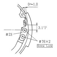
Adjust aperture diameter so that the position of aperture lever #23 comes within standard value of  $3.1^{+0.1}_{0.0}$  by unfastening screws #76×2 at full aperture. Adjust the gap between bayonet and #23 be 0 to 1.0mm.
