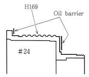
\*Apply grease H169 to two portions in the groove for keys #22×2.
