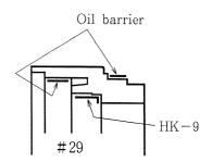
**Note:** You can use grease (FC-4) to substitute grease (H169 and HK-9). The effect of the grease is not guaranteed under the low temperature environment (-20°C). Be absolutely sure to use grease (H169 and HK-9) under the low temperature conditions.
