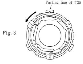
As shown in Fig. 2, screw in #24 fully and rotate the ring in the direction indicated by an arrow so that the projection of #24 comes in the middle of the projections of #25. (Refer to fig. 3)
