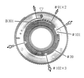
\*Attach #101 so that the stopper of aperture lever comes to  $3.1^{+0.1}$ .
