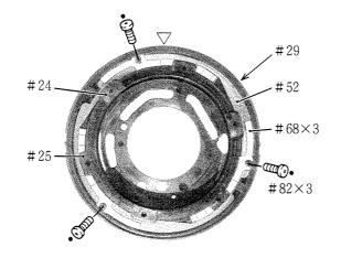
Mount helicoid rings #24 and #25 on #29 with washer #52, leaf springs  $\#68\times3$ , and screws  $\#82\times3$ .
