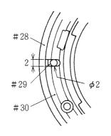
Aligning the 2mm width groove of bayonet mount and  $\phi 2$  hole of #29, fasten the bayonet mount with screws #71 and #72×2. Mount the screw #71 (black) under the index.
