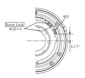
Unfasten screws #152×2 to adjust the position of the aperture lever #23 so that it comes into the rated value of  $3.1^{+0.1}_{0.1}$  to bring the aperture diameter whitin rated value at full aperture.
