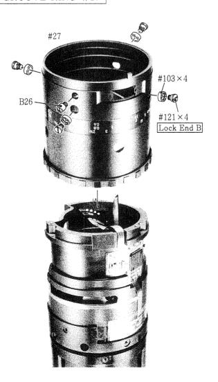
• Apply the grease G92KA to each lead groove and the gear area inside the lead groove barrel #27.
