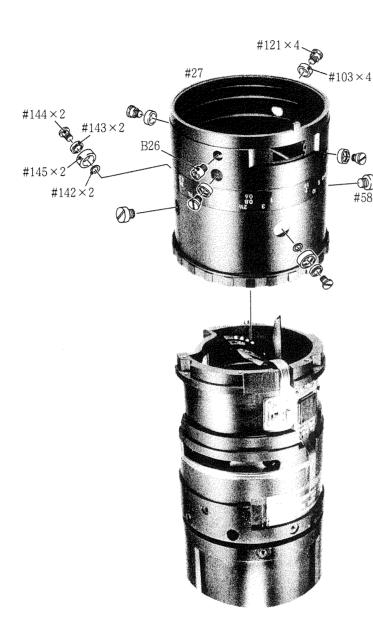
• Rotate the lead groove barrel #27, let the hole position to meet each guide roller to remove them.
