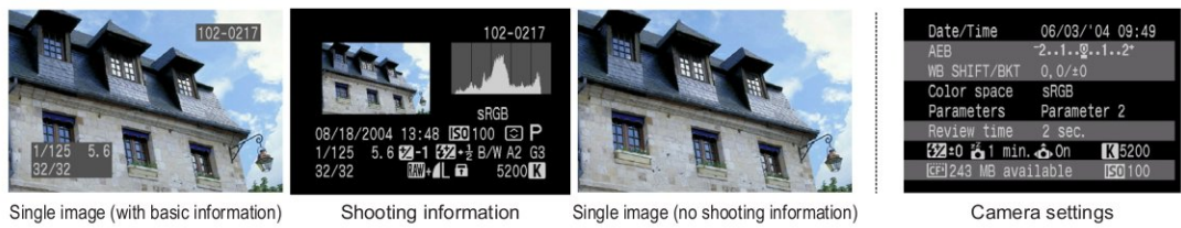
Fig. 030 Single image display/Shooting information/Camera settings
