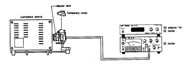
e SS adapter for EE tester • EE tester e Luminance source · Camera to be measured e Master lens K value dial: 1.3 F dial: 5.6 K value : 1.3 : 100 Focusing ring: ∞ ASA dial : 100 EV dial: Same as luminance Luminance : See Exposure mode: A : See source. Table below. Aperture Table below. Exposure adjustment: 0
