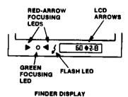
The lens remains at the focus setting as long as you hold the release button partially depressed. You can then compose the picture the way you want it; to change the focus, let up and redepress the release button part way. Fully depress the release button to release the shutter.
