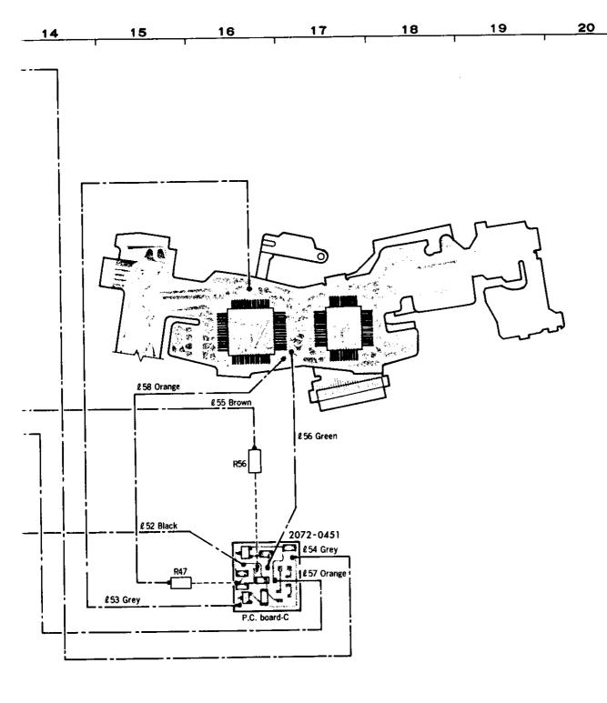
■ Lead wires (shown by alternate long and short dash line) and PC board-C set (0451) are discontinued in step 3.\*
