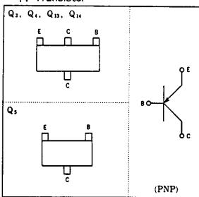
Check conductivity between the terminals of B, C, E.
