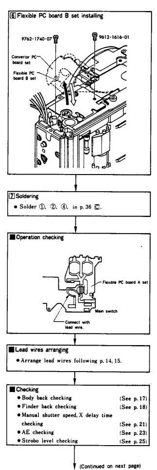
Place flexible PC board B and convertor PC board set in position and tighten screws (9762-1740-07)(9612-1616-01).
