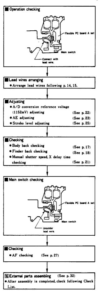
Check\* with main switch connected by lead wire.
