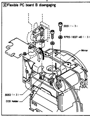
Pushing CCD holder (the area shown by arrow), remove screws (5051×3) and washers (9795-1837-40×3) by the use of hexagon wrench......Pay attention NOT TO TOUCH THE MIRROR.
