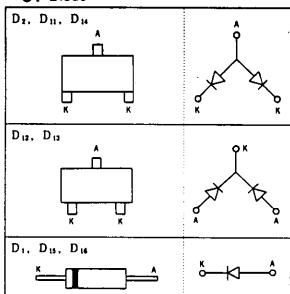
Check conductivity between the terminals of A, K.
