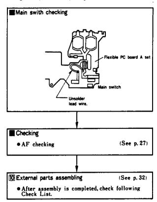
Remove the lead wire which has been soldered for function checking.
