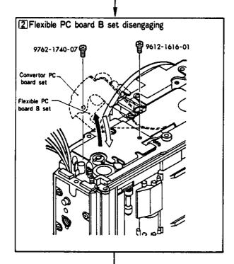
1. Remove screws (9762-1740-07)(9612-1616-01) and then lift up flexible PC board B and convertor PC board set as shown.
