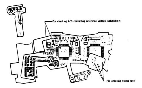
VR1: for adjusting A/D converting reference voltage
