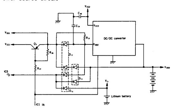
With battery holder attached, battery power is supplied to each IC as  $V_{DD0}$  and  $V_{DD1}$ . By turning metering Sw. ON  $\rightarrow$  IC  $_1$  6 becomes at L  $\rightarrow$  Q $_5$  ON  $\rightarrow$  DC/DC converter is activated, stabilized power is supplied (as  $V_{CC1}$  and  $V_{DD1}$ ) Output of  $V_{CC2}$ .
