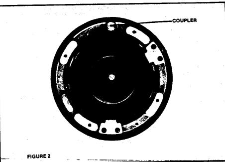
the aluminum helical ring (fixed ring). Then back out the outer helical ring 1¼ turn (CCW as seen from the front).
