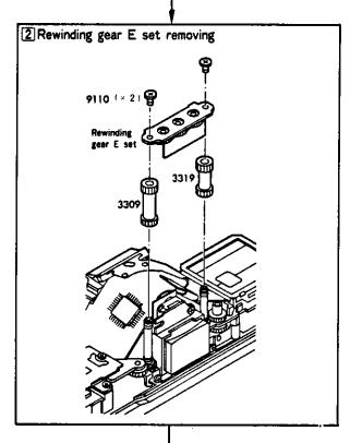
1. Remove two screws (9110), rewinding gear E set, 3309, and 3319.
