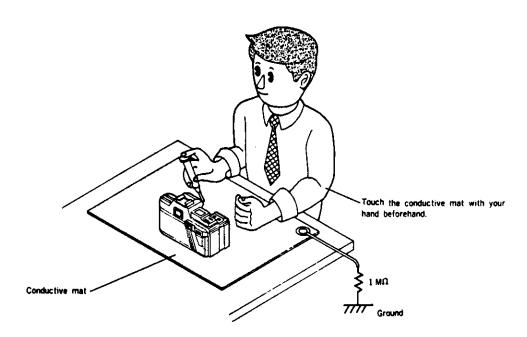
■When grounding is impossible, connect the cable to a large metal plate (steel desk or shelf).
