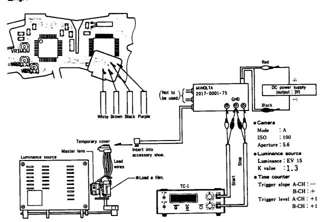
2. With the shutter released, adjust by turning VR<sub>3</sub> so that the indication of the time counter is  $0.45\pm0.06ms$
