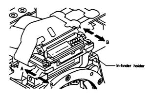
• After adjusting, tighten screws and check in-finder display position.
