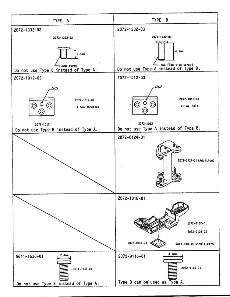
For parts of A type which cannot be supplied, (X) is attached to the tail of the part number in the table. If it is necessary to modify the (X)-marked part, replace it with B type.
