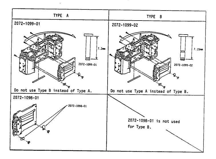
For parts of A type which cannot be supplied, (X) is attached to the tail of the part number in the table. If it is necessary to modify the (X)-marked part, replace it with B type.
