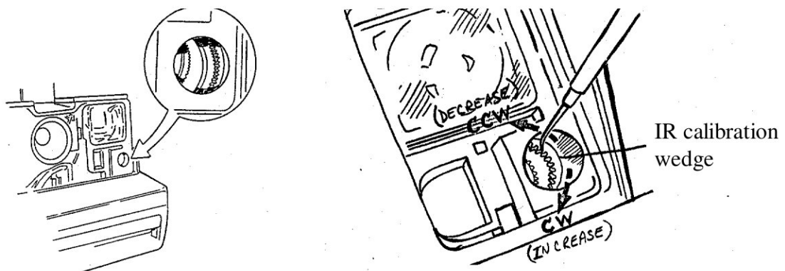
Fig. 6 Adjusting IR Calibration Wedge
