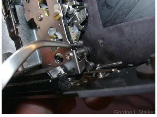
This is the actual opening shutter latch, shown in the cocked position. This is operated by the
