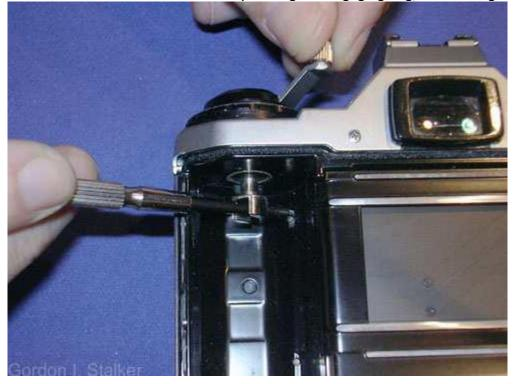
Do not remove the rewind shaft unless you intend to remove the back at this point. Closing the back without the rewind shaft makes it very difficult to release the latch. To make sure you do not close the back inadvertently you can remove the back by sliding the screw shown below down.
