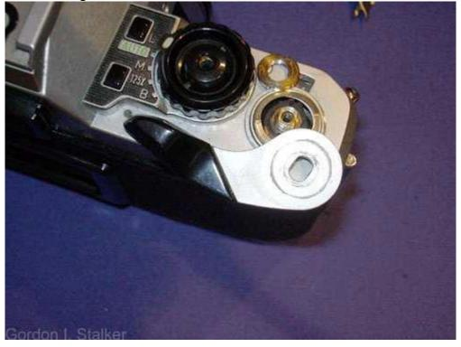
The release button should not normally need to be removed, but if you do need to remove it then proceed as follows. If not skip to removing the rewinder. Using an improvised tool unscrew the collar around the release button. (This is often quite loose!)
