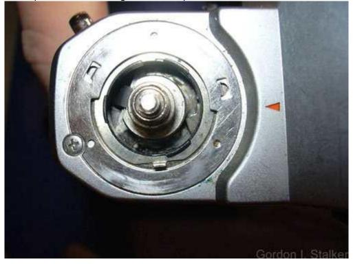
Now remove the two screws on top of the cover. They are slightly different right and left.
