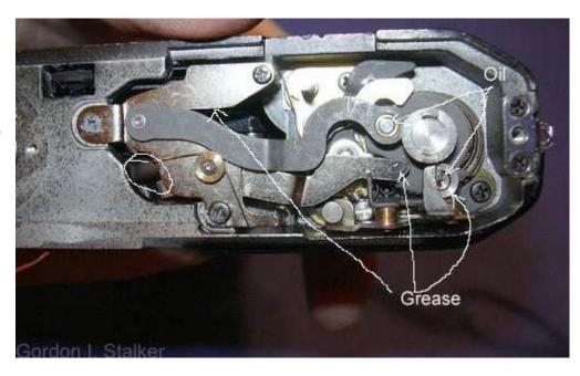
This is the mirror cocking lever, shown in discharged position. The mirror is in it's resting position.
