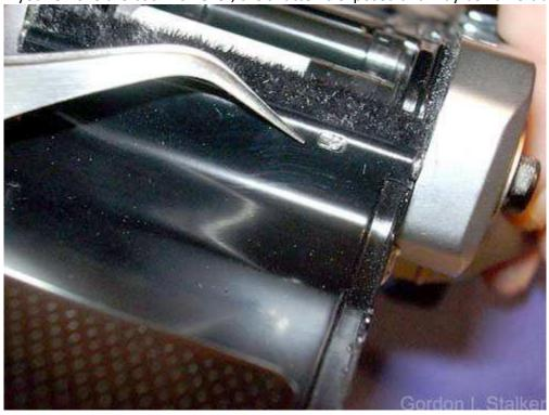
Removing the winder exposes the film speed selector retaining nut. This is conventionally threaded.
