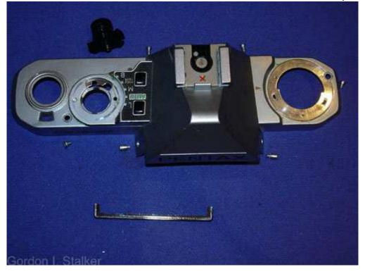
Detailed below is part of the film counter mechanism. You probably won't need to disassemble this unless someone has forced a jammed camera, but the hair-spring indicated, is easily dislodged from the groove ringed whilst working on the camera. Which is what has
