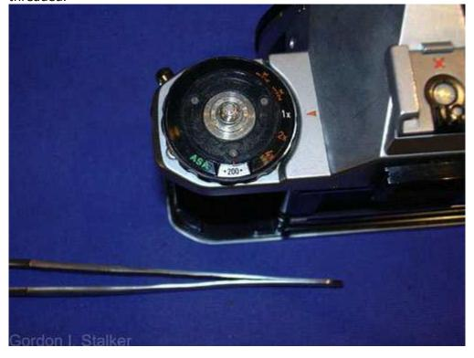
Before removing the selector dial, it is useful to set it to a default position as shown in this example.
