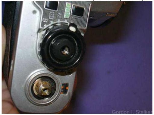
Remove the mode selector knob. Note the little pin beside the 'AUTO' setting. This needs to
