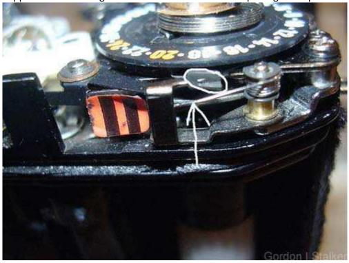
If you have removed the top to adjust shutter speeds or the LED display, the two presets adjust each as labelled. Note that the PCB they sit on is a ceramic component. Cracks in this
