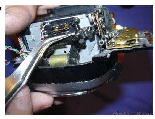
Pushing this lever forward primes the mirror, and reveals the straight mirror lifting spring.
