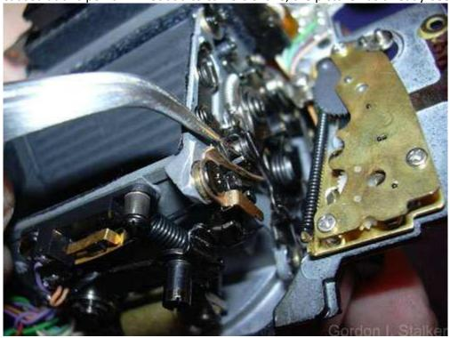
This lever is operated by the mirror lifting arm, and is responsible for releasing the opening curtain just after the mirror comes to rest in it's upper position. There is a slight delay between releasing the shutter latch and the curtain opening so that the mirror is sure to be out of the way before it opens. This means that the latch actually operates just before the mirror is fully up, the rest is down to the delay.
