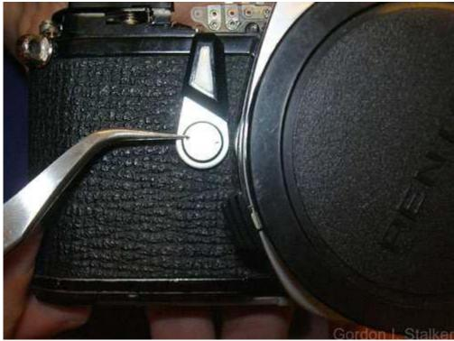
The Leatherette can be carefully peeled off. Start the edges with a dental probe. Note the mechanism showing through the hole. This is the shutter release arm. It should not require
