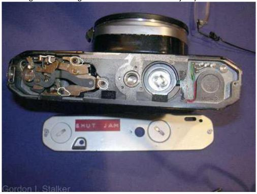
Two important plastic items released by removing the bottom cover. Make sure these are kept safe.
