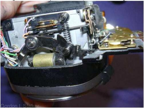
This is the body-mounted release lever operated by the shutter release button, and the timer release escapement. It bears on the upper arm of the mirror release latch.
