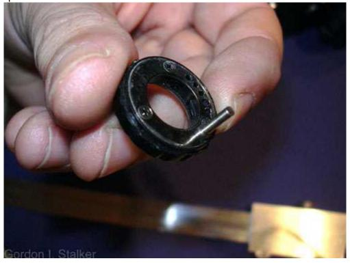
The pin should be removed carefully, there is a tiny spring below it which could get lost.
