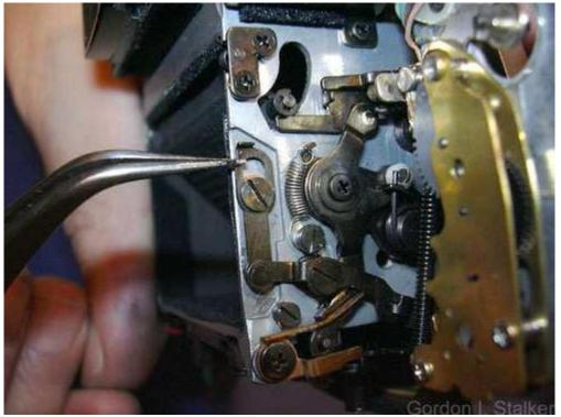
Note how the forked end locates into the spring release.
