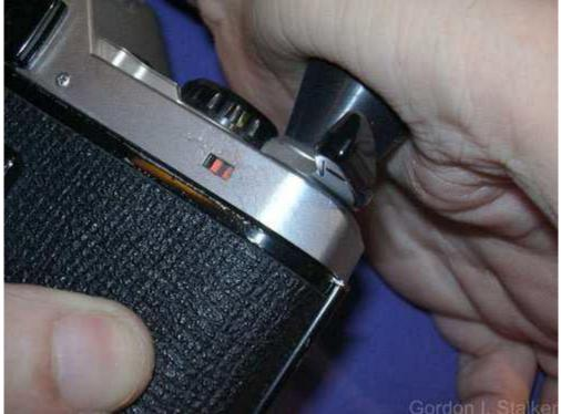
This exposes the retaining nut. This is also left-handed, and may be removed with an improvised tool.
