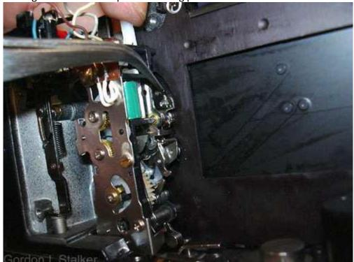
More details on the shutter can be found in my page on the Pentax M series shutter. The cocking mechanism can be lightly lubricated as shown. The lubricants here are not critical, but it is as well to use oil recommended for cameras (or watches), as this will be formulated to ensure long life and correct lubrication at a wide range of temperatures.
