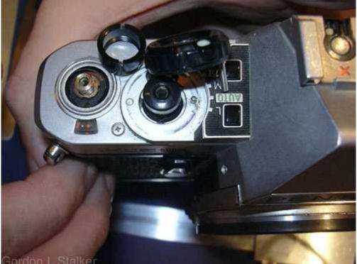
The mode selector has a long shaft which engages with a cam to select the mechanical speeds.
