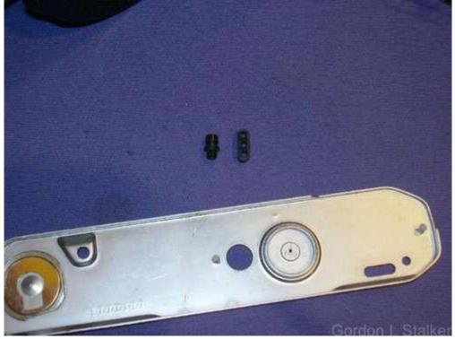
The leatherette trim should now be removed. To do this first remove the self timer lever. The retaining screw is left handed, and can be removed with our improvised tool. There are a number of washers underneath.
