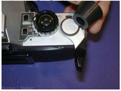
Apply pressure firmly with the ball of the thumb. If this does not loosen the cap, use a small piece of self amalgamating tape to increase friction. If that fails you should obtain (or make) a 16mm flexiclamp. Alternatively, if you are prepared to spend three-quarters of an hour cleaning it off with a wooden scraper, glue the bung onto the cap with superglue!
