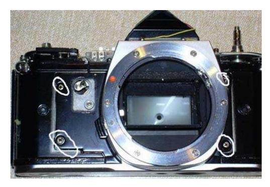
Remove the lens standard complete with mirror cage, prism, and electronics. Lift the assembly about 5mm to disengage the cocking mechanism, and withdraw forwards.
