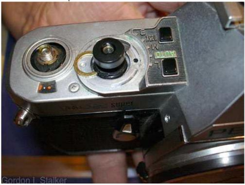
The rewind crank can be removed by locking the engaging dog, and turning the crank.
