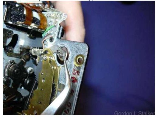
The lower arm of the mirror release latch holds the mirror lifting arm in the mirror resting position. The mirror return spring is under considerable tension at this point, which is a good reason for making sure that the camera is not left in a primed state. Leaving a spring in a stressed state for long periods can weaken it.
