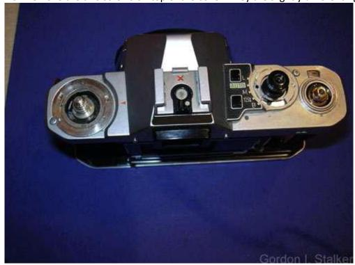
The two screws here should be removed.
