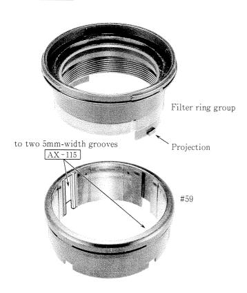
• Modify Shift ring #59 and insert the projection of the filter ring into a 5mm-width groove (with grooves on both sides) on the shift ring.
