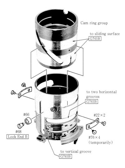
**Inspection:** Check operation by rotating the cam ring #50.
