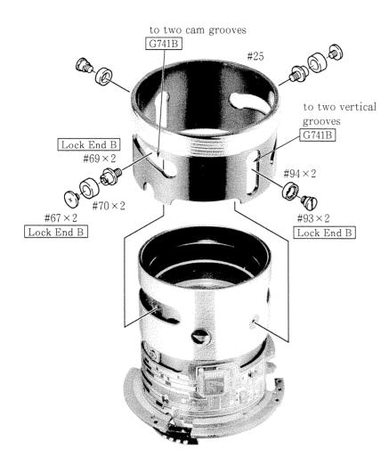
**Inspection:** Check operation by rotating the cam ring #50.
