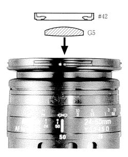
• Attach the retaining ring #42 using tool J11239.
