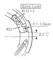
• Unfasten screws #112×2 to adjust the position of the aperture lever #23 so that it comes into the rated value of 3.1<sup>-0.1</sup> to bring the aperture diameter within rated value at full aperture (f/3.3). Together with this, adjust the gap between bayonet mount and aperture lever #23 be 0mm to 1.0mm.
