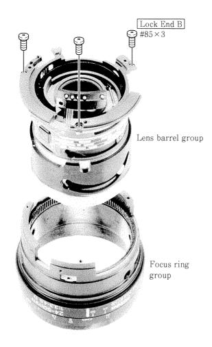
**Inspection:** Rotate the focus ring to check operation of AF gear. If it does not move properly, adjust the AF gear attaching position.
