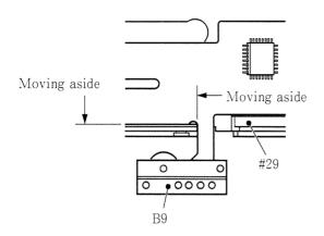
• Attach the AF contact FPC unit B9 on #29 by moving it aside as shown in figure.
