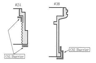
• Wrap tape TA-0012 around to secure helicoid ring #24 and filter ring #38.
