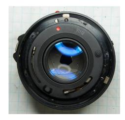
The rear cap is removed by turning it clockwise until the first lump lines up with the release button.
