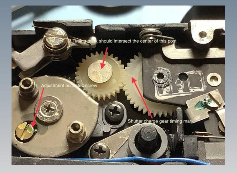
I wanted to take a moment to show the shutter charge gear timing and if you look closely you can see why the adjustment is too much resulting in a "less than positive feel" as I mentioned in the first post during the camera checkout procedure...
