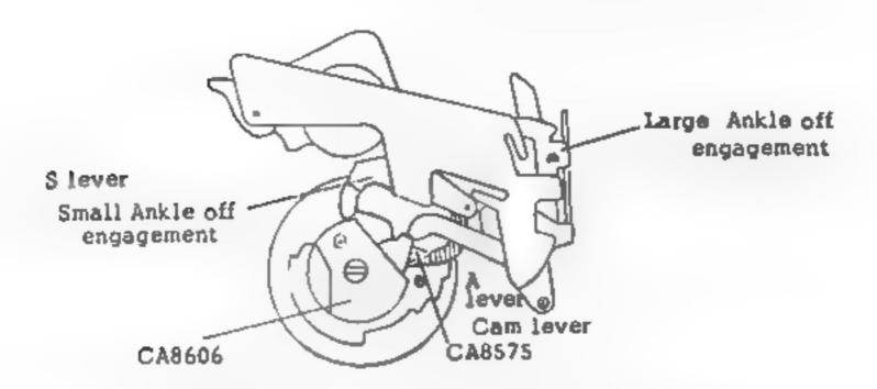
Both the Sankle and the Lankle are released from engagement by the Slever and the Alever.
