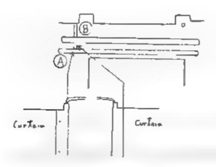
Make fine adjustment on the alignment of the Patch of 8600 and the Scratched-Line on the die-cast by adjusting the 5 holes' positions.
