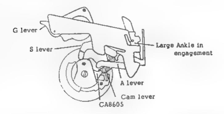
The A lever is released from 8605 and the Lankle is engaged. The S ankle remains off engagement by the S lever. To differentiate shutter timing for 1/1 and 1/2, the message is transmitted from 8575 to the Cam lever and the operating angle of the G lever will be changed.
