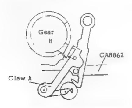
(2) Press 9078, let Claw A of 8567 engage onto the Gear B, and see if there is a space of 0.2mm or above between 8810 (Plate) and Claw B when the spece between the obiong hole of 8862 (Plate) and 8864 (Shaft) gets to 0.8mm. If there is not, an adjustment should be made by bending the portion marked with a circle in the picture below.
