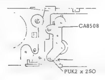
In case where the Shaft rattles vertically due to deformation of 8508, insert a U washer (0.1 - 0.2) underneath the Plate R on the arrowed side.
