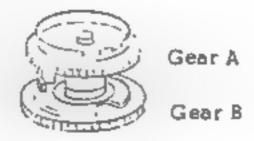
(4) Do not change the position of the Gear B but turn 8520 until the Patch of 8600 (Curtain) reaches closest to the Scratched line ((A below) on the Die-cast Body. Then raise (8520) and let it engage onto the Gear B.
