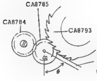
The clearance between boss of 8785 and 8793 should be over than lum.
