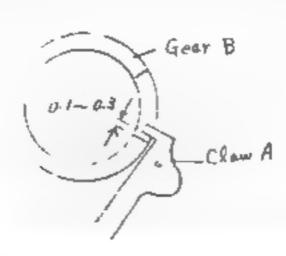
When Claw A is shaken if its lower edge hits the Gear B, an adjustment may be made by bending the Plate (B).
