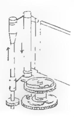
1st curtain stops at the improper position.
