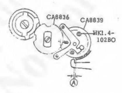
Prior to film advancement, when the Gear A is pressed in the arrowed direction, the distance between 8840 and the Gear A should be -0.10 ~+0.3. (-0.10 means the state where the Gear A comes in contact with 8840 and further moves by 0.1.)
