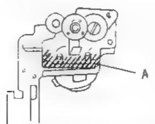
To be cleaned and applied with Oilproof Liquid.
