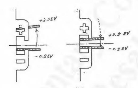
o When the lens aperture is stepped down from the wide open state, the meter needle should once swing down to a position lower than -0.5EV before it is stabilized at +0.5EV. (See Fig. B.)
