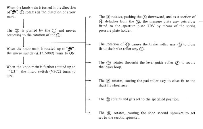
The 6, connected to the 4, rotates, causing the first sprocket shoe to get set to the first sprocket, then the 7 gets released from the upper loop, and the upper loop is secured.
