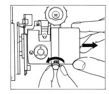
3 Remove the halogen lamp from lamp socket and insert a new lamp to the socket.
