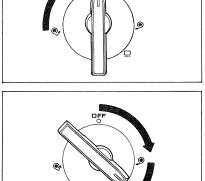
Note: (1) When the master control knob is set to from OFF, the TRV-16 may start rewinding after a few seconds' pause depending on the film volume on the reel to be rewound. This is not a fault but a safety mechanism for rewinding. The TRV-16 is designed to increase motor torque gradually for the protection of film.
