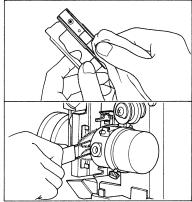
4 After cleaning, align the two pins at the upper and lower parts of the pressure plate holder with the corresponding slots on the pressure plate base and push it back.
