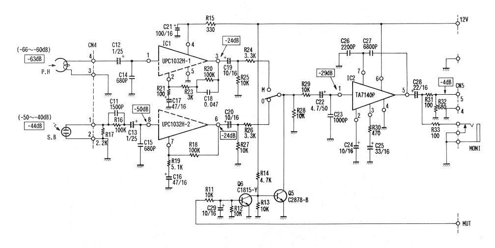
V- 4 SCHEMATIC DIAGRAM FOR AMPLIFIER (E44112)
