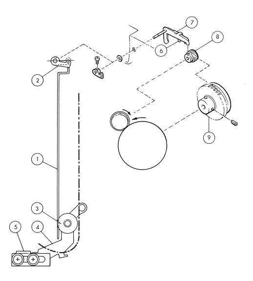
When there is no more loop at the bottom of the film gate, the film pushes ① up, causing ② to move upward (in the broken line direction) and ⑧ to get detached from the claw ⑥. In the meantime, ⑦ provides rotation to ⑧, and ⑧ rotates due to ⑨, causing ③ to get pushed downward to form appropriate loop. The ⑧ takes 1 turn before being stopped by ⑥.
