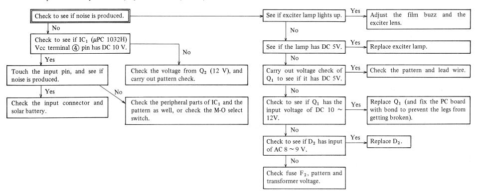
\* Failure in reproduction of magnetic sound (optical sound being normal):
