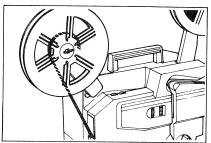
3 Make sure that the film is properly loaded through the channel by turning the take-up reel clockwise by hand to observe free movement.
