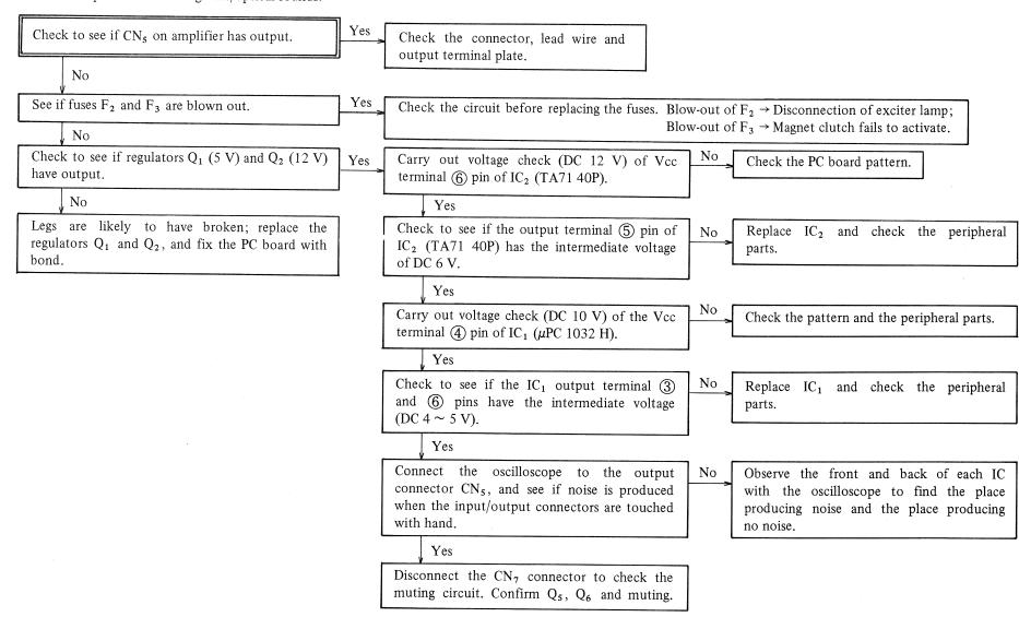
\* Failure in reproduction of optical sound (magnetic sound being normal):
