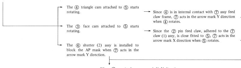
When  $\bigcirc$  acts in the arrow mark X, Y directions, the  $\bigcirc$  feed claw also activates to feed the film.
