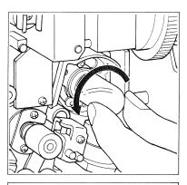
2 To replace the exciter lamp, align three prongs on the socket with the holes on the lamp flange and turn the lamp head clockwise until it locks into place.
