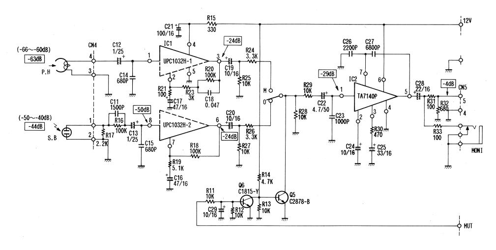
SCHEMATIC DIAGRAM FOR AMPLIFIER (E44112)
