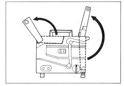
3 Install the feed reel with film, facing the film perforations toward yourself, on the feed reel spindle, and turn down the reel lock to secure the reel.
