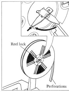
4 Install the supplied 800 ft (240 m) take-up reel, which is stored on the rear of the TRV-16, or an optional reel of more than 800 ft (240 m) film capacity on the take-up reel spindle. Be sure to lock the reel by using the reel lock. The reel capcacity is max. 2000 ft (600 m).
