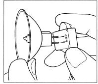
4 Install the lamp and then put the lamp holder and fix it with the screw.
