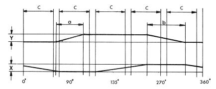
X: Surface cam Y: Triangle cam a: Back feed
