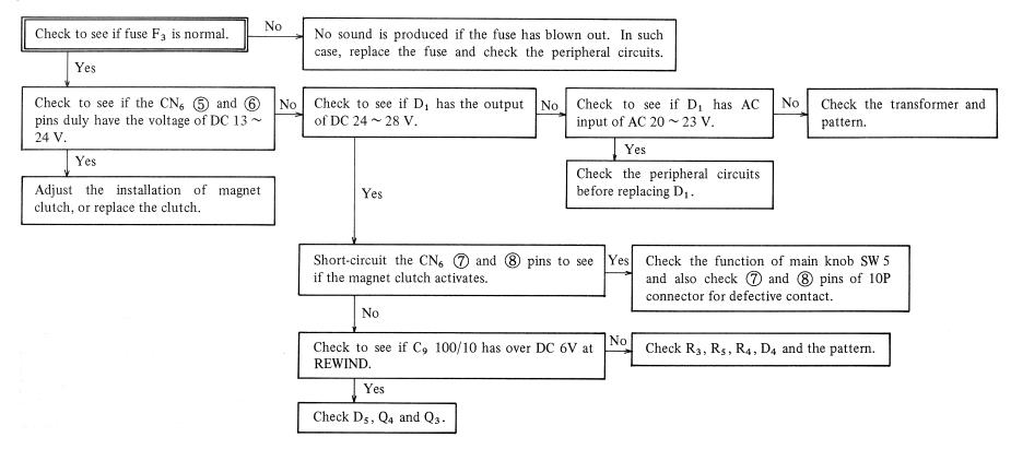
\* Magnet clutch has excessively small initial power for activation:
