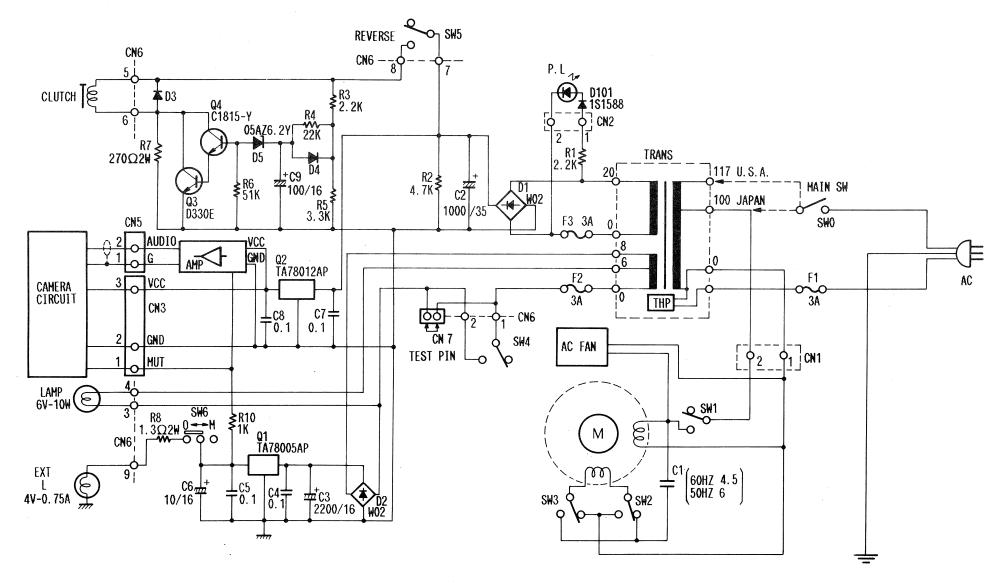
SCHEMATIC DIAGRAM FOR MACHINE (E44113)
