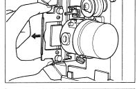
3 Clean the aperture and the pressure plate with the supplied brush and a soft lint-free cloth.
