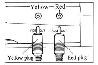
2 Connect the yellow plug to VIDEO IN and the red plug to AUDIO IN receptacles of a monitor TV respectively.
