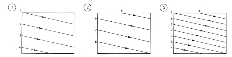
In CCD, this interlaced scanning is taken into consideration, and the photographic signal charges are read out.
