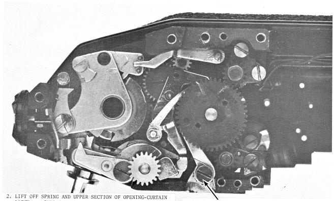
2. LIFT OFF SPRING AND UPPER SECTION OF OPENING-CURTAIN LATCH - - PULL OUT LOWER SECTION OF OPENING-CURTAIN LATCH TOWARD BOTTOM OF CAMERA.
