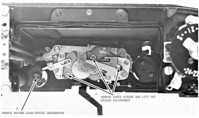
REMOVE TWO SCREWS AND RETARD-CONTROL-RODS BRIDGE
