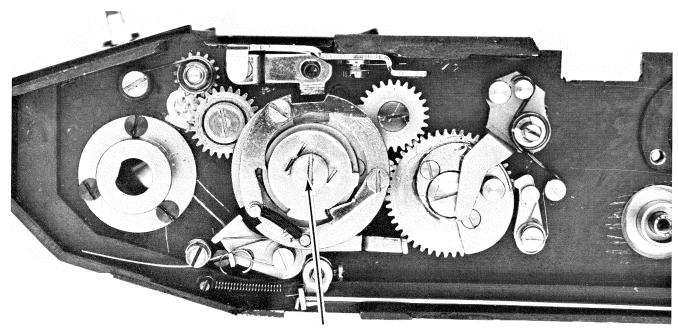
REMOVE SCREW AND LIFT OFF OPENING-CURTAIN CAM
