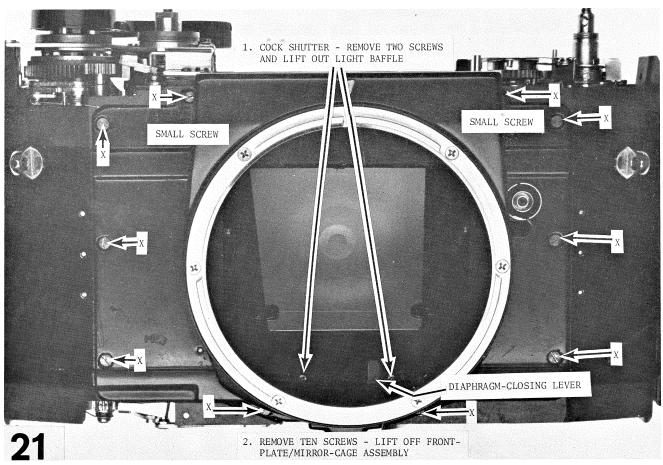
2. REMOVE TEN SCREWS - LIFT OFF FRONT-PLATE/MIRROR-CAGE ASSEMBLY
