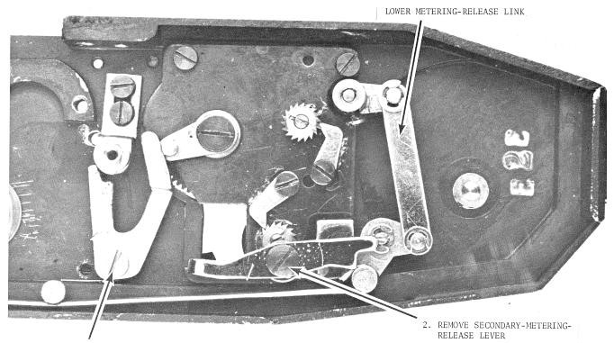
1. REMOVE DIAPHRAGM-CLOSING-LEVER LATCH
