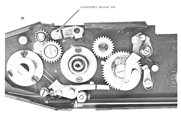
1. REMOVE SCREW AND LIFT OFF COUNTER DIAL (RETURN SPRING IS UNDERWEATH COUNTER DIAL)
