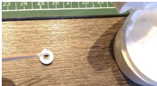
The shutter latch is lubricated with silicone grease.
