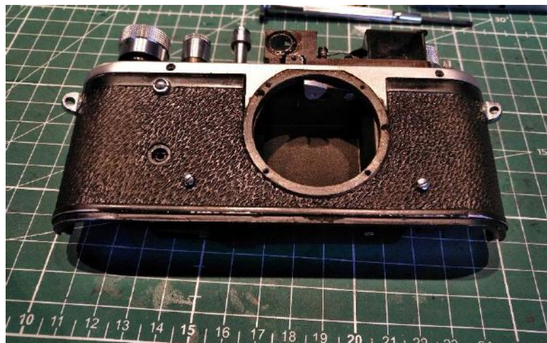
Shutter crate secured to the body.
