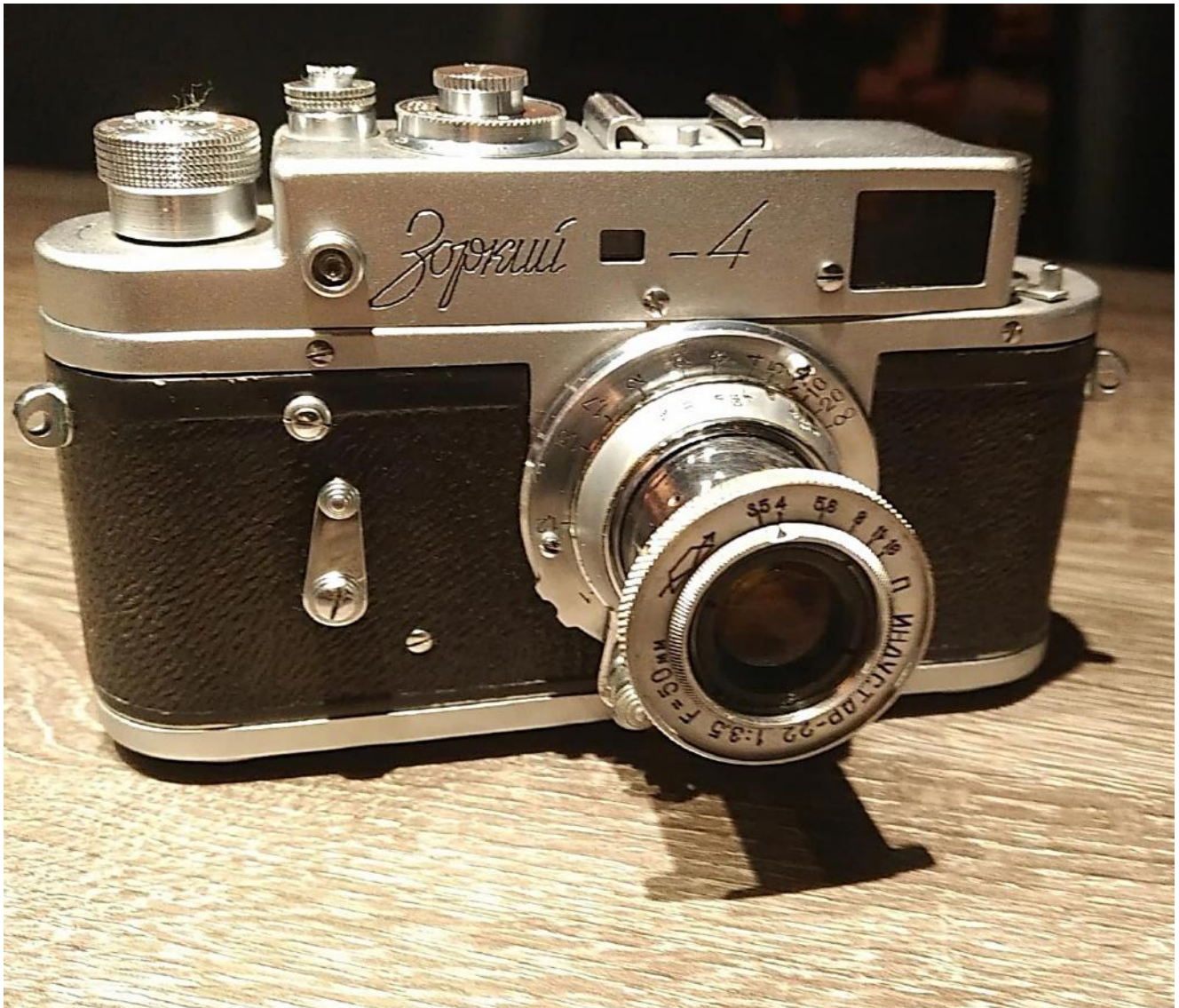
1961 Zorki-4 with Industar-22, retractable, 50mm f/3.5 lens.
