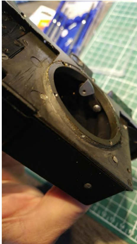
Cleaned lens mount base.
