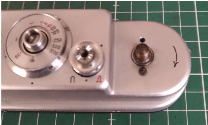
Securing the two screws above and below the rewind shaft.
