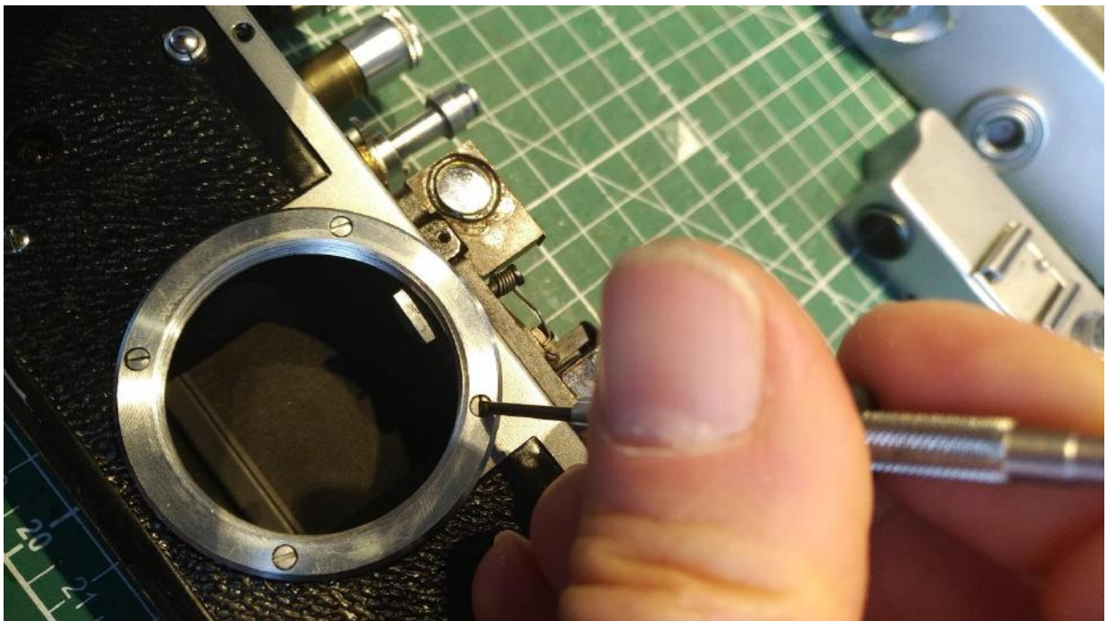
Taking out the lens mount.
