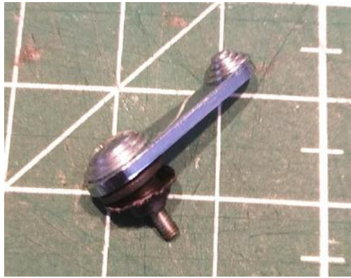
Self-timer lever with light seal taken out.
