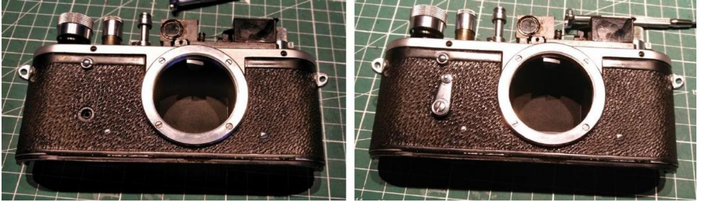
Reattaching the self-timer lever.
