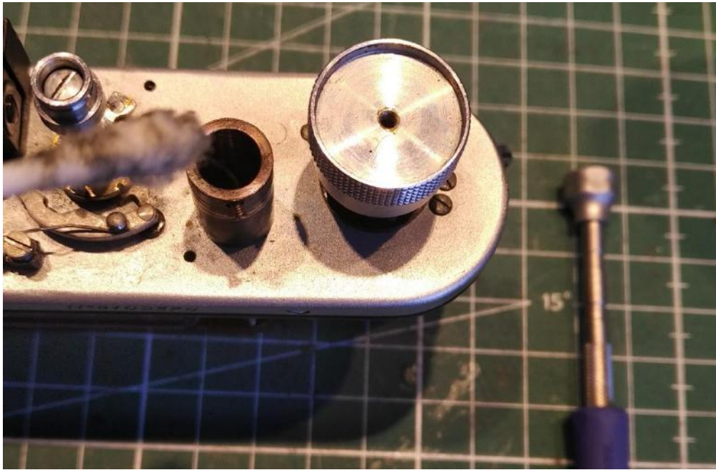
Cleaning the shutter-rewind mechanism shaft.
