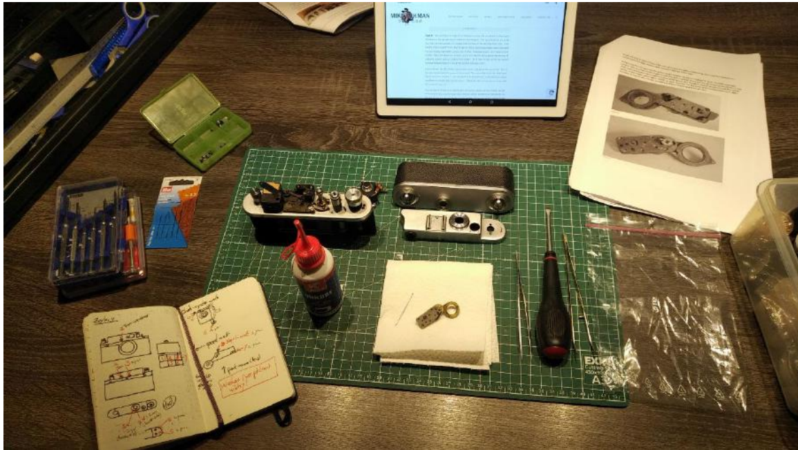
Degreased slow-speed-mechanism, ready for lubrication. Note that I have all references mentioned in the Introduction strategically lying around.
