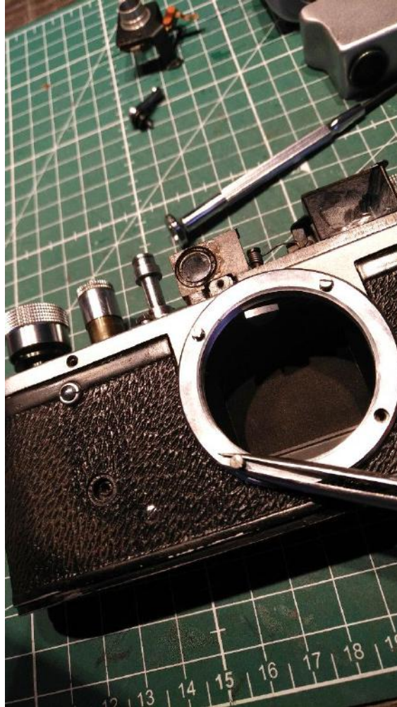
Using a pair of tweezers may aid in attaching the lens mount screws.
