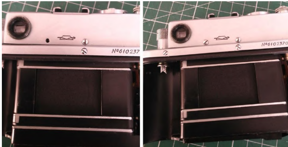
Securing the top on the back using two (non-identical) screws.
