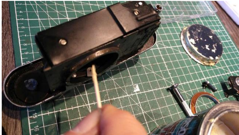
Applying glue to the rim of the lens mount base.
