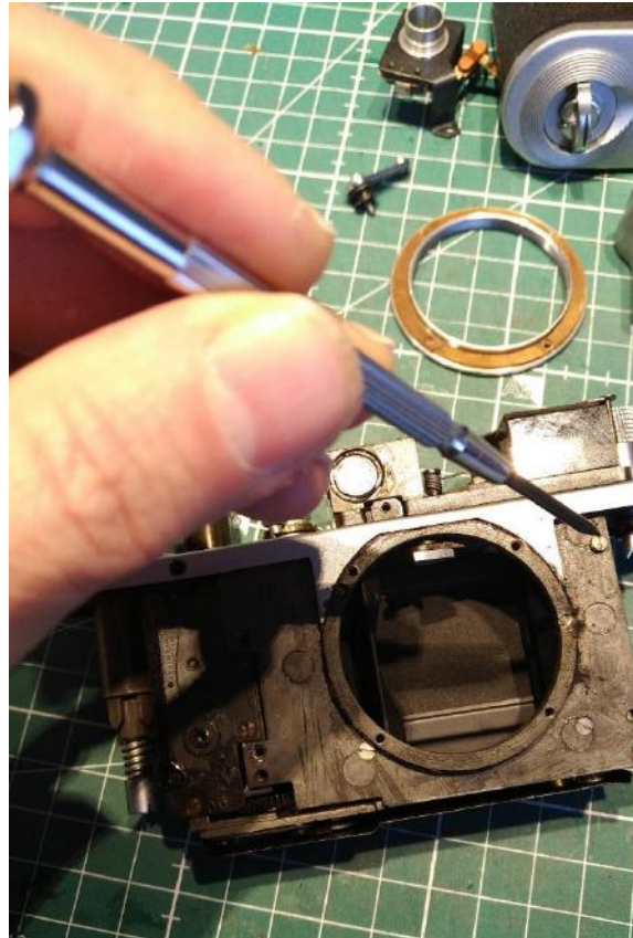
Securing the front of the shutter crate.
