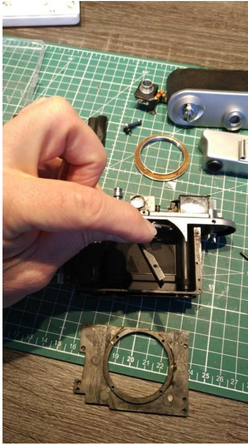
Replacing the light baffles. Don't worry too much about the exact placement.
