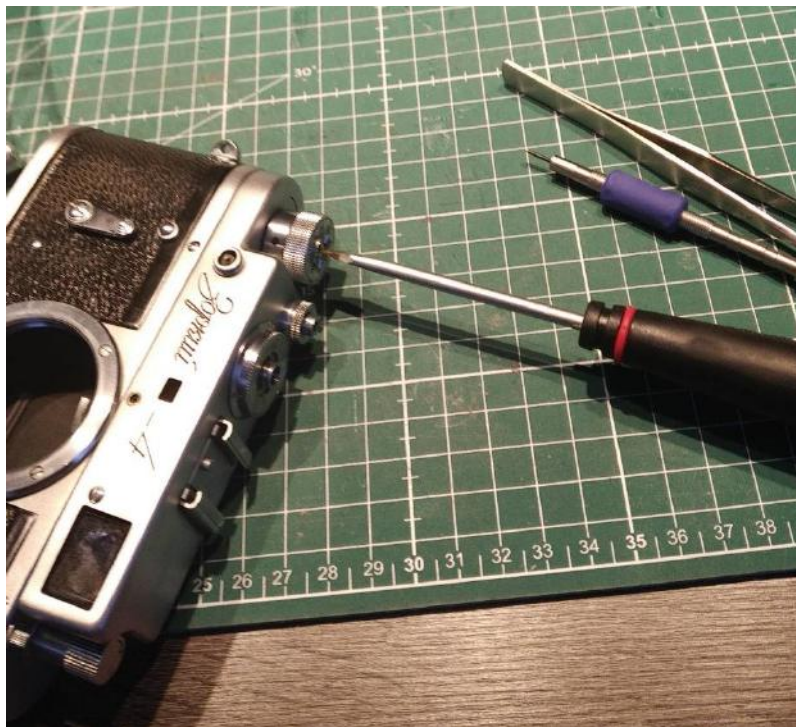
Removing the Zorki-4 winder knob top plate.
