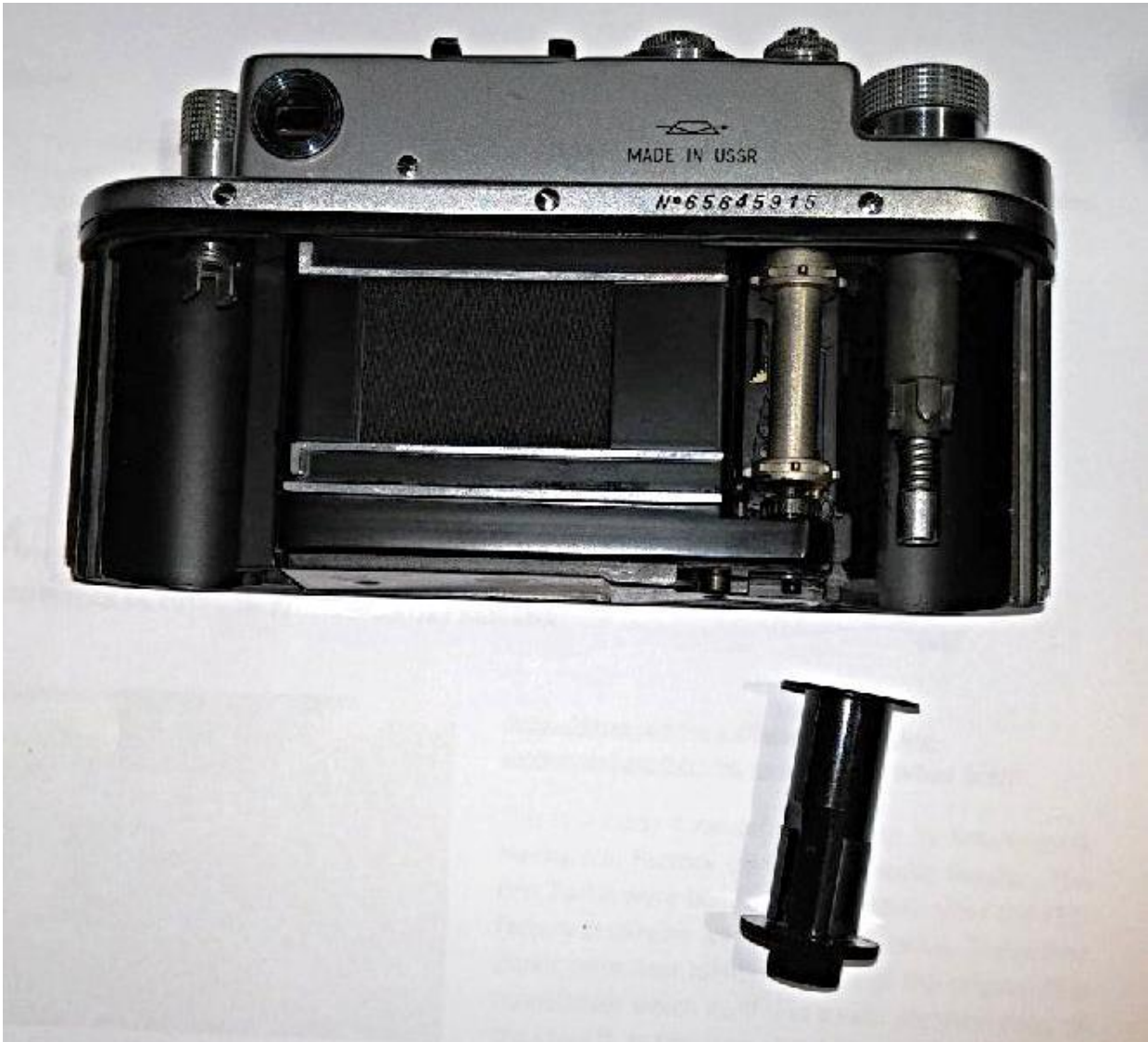
1965 (see serial number) export - ('made in USSR') Zorki-4 with take-up spool.
