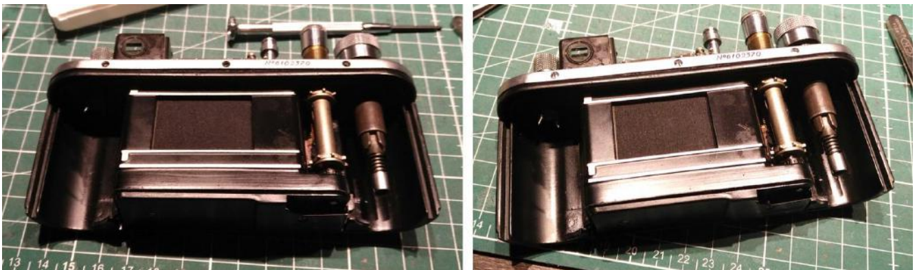
Securing the top plate to the body on the back.
