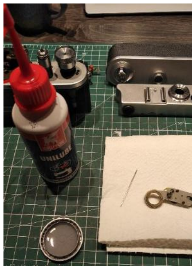
Lubricating, using sewing machine oil and a needle. The lid of a 35mm film container forms a handy oil reservoir.
