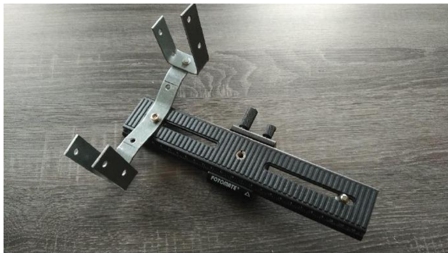
Rig to hold the Zorki-4 camera at one end.
