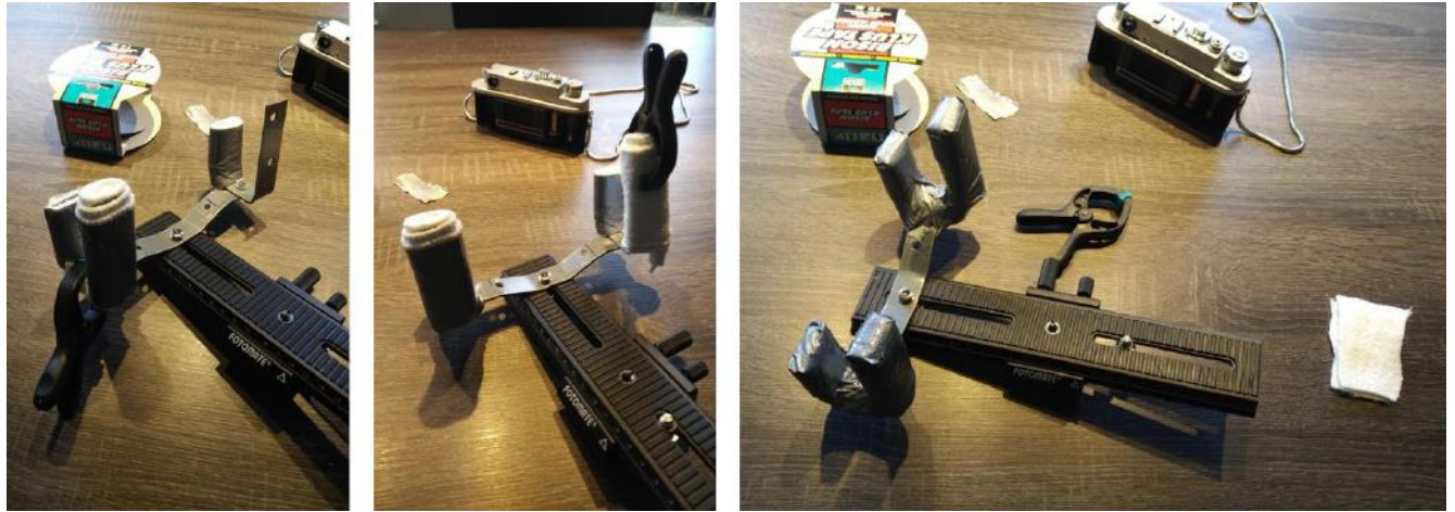
Making cushions to hold the Zorki-4 without scratching it.
