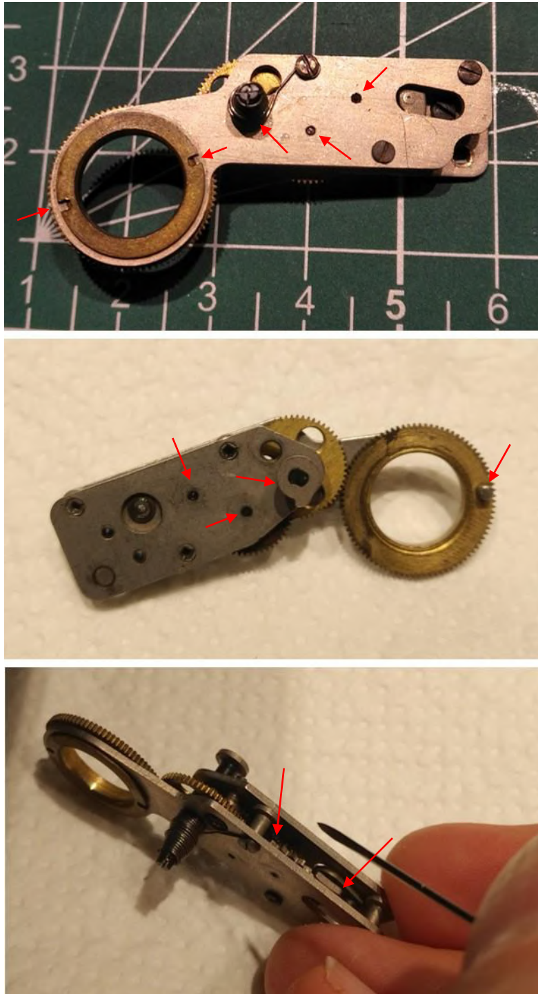
Lubrication points for the slow-speed-mechanism (red arrows).
