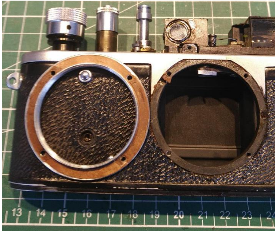
Shims underneath the lens mouth.
