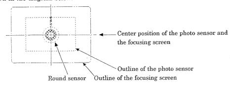
[ Reference ] If a lens with a large aperture (ex. FA 50mm f/1.4) is mounted on the body, the pattern of the photo sensor will be seen easily on the mirror.
