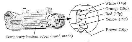
2) Install a temporary bottom cover and a battery cover, set the battery to the body, and install the power SW adapter to the release socket.
