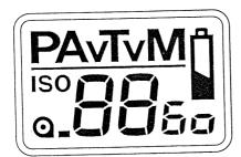
P: Programmed AEAv: Aperture-Priority AETv: Shutter-Priority AEM: Metered Manual Mode
