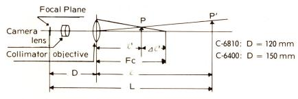
D = Distance between collimator objective and film plane
