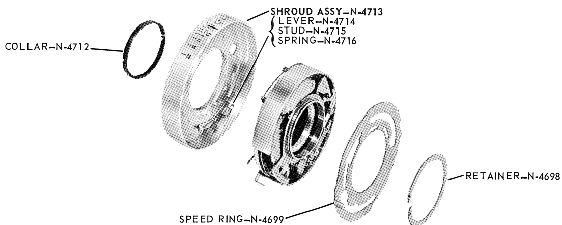
FIGURE 28. LENS MOUNTING PLATE ASSY-N-4691
