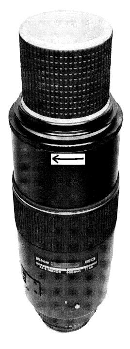
• Rotate the focus ring to the infinity side and set the end of the assistance tool of wrench (J11296) to the notch of the frame for the 3rd lens group to attach it. Then, rotate the screw ring in the arrow direction to fix it.
