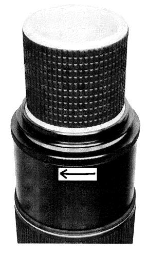
Rotate the focus ring to the infinity side and set the end of the assistance tool of wrench (J11296) to the notch of the frame for the 3rd lens group to attach it. Then, rotate the screw ring in the arrow direction to fix it.
