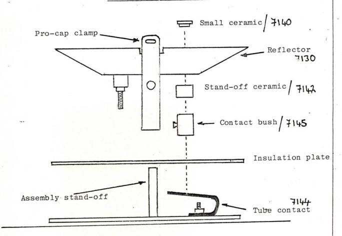
A complete tube assembly is available comprising of flach tube, reflector, ceramic stand-offs and bushes. Part numbers are as follows:-
